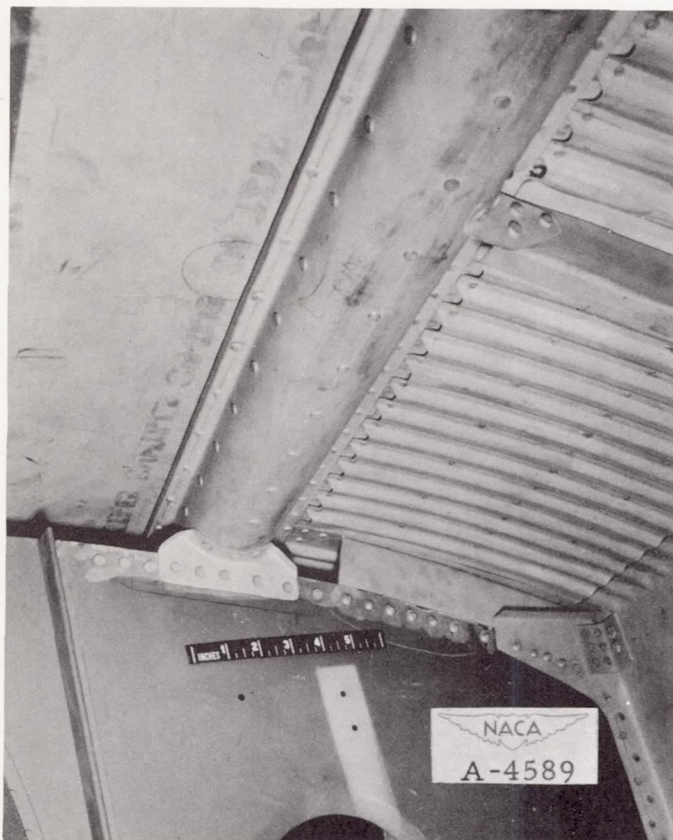
Figure 6. - Typical details of attachment of revised wing outer-panel leading edge to original structure.
