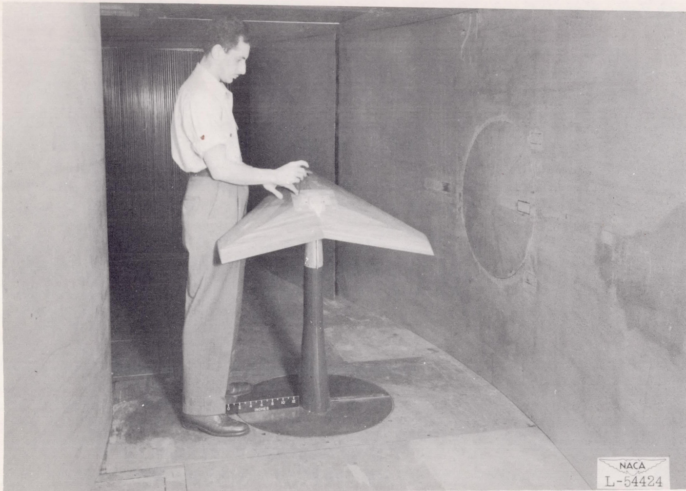
Figure 2.- Photograph of wing having taper ratio of 0.25 mounted in curved-flow test section of Langley stability tunnel.
