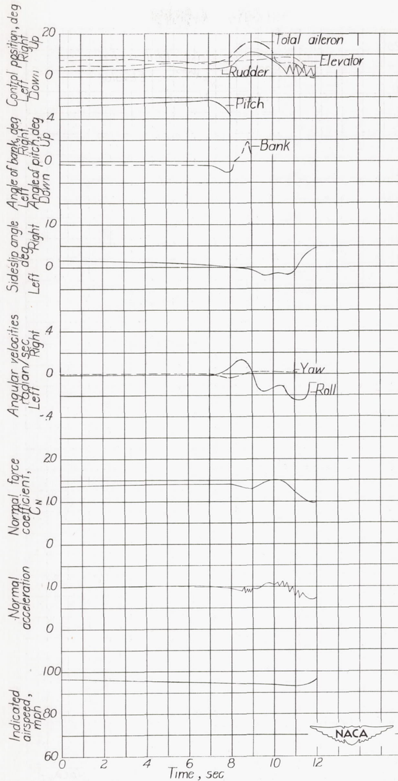
Figure 15.- Typical time history of a stall. Fighter-type airplane. Gear and flaps up; canopy closed; propeller idling; altitude, 7000 feet.
