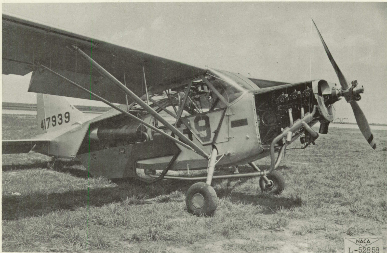
Figure 8.- Muffler installation in modified test airplane.
