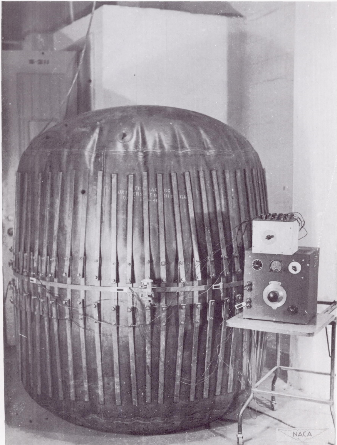
Figure 48.- Pressure bag used to load ring. (Uniform load could not be obtained.)
