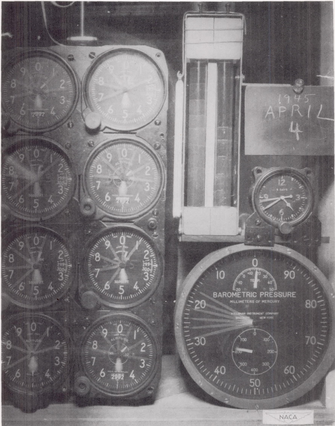
Figure 3.- Photographic observations in primary dynamic calibration. Rate of ascent, 30,000 feet per minute.
