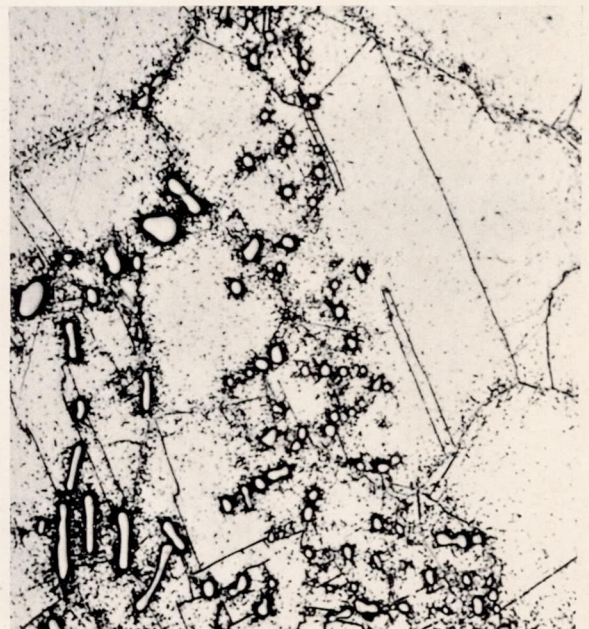
(b) Disc NR-74B-QA; radial section near rim of disc in center plane. Electrolytic sodium cyanide etch. Disc treatment: 2300° F water-quenched; 16 hours at 1400° F.
