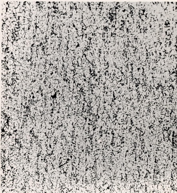
(b) Specimen 2X; 1872 hours at 1350° F under 15,000 psi.
