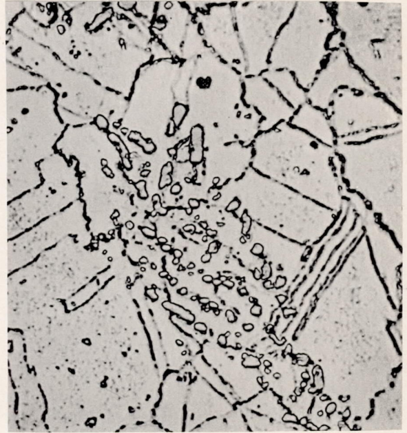
(a) Specimen 13X; 1002 hours at 1200° F under 35,000 psi.
