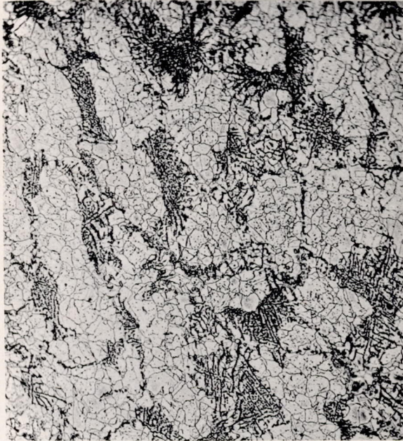
(a) Specimen 13X; 1002 hours at 1200° F under 35,000 psi.
