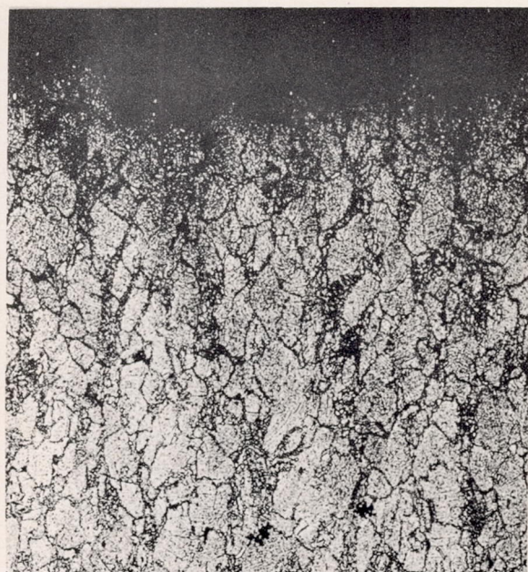
Fracture - 100X Interior - 1000X (b) Specimen 14Y; 951 hours for rupture at 1350° F under 25,000 psi.
