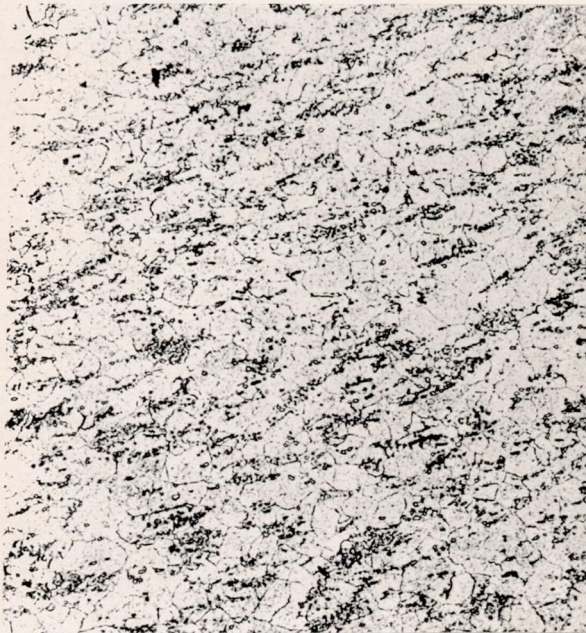
(c) Specimen 4X; 2136 hours at 1500° F under 12,000 psi.
