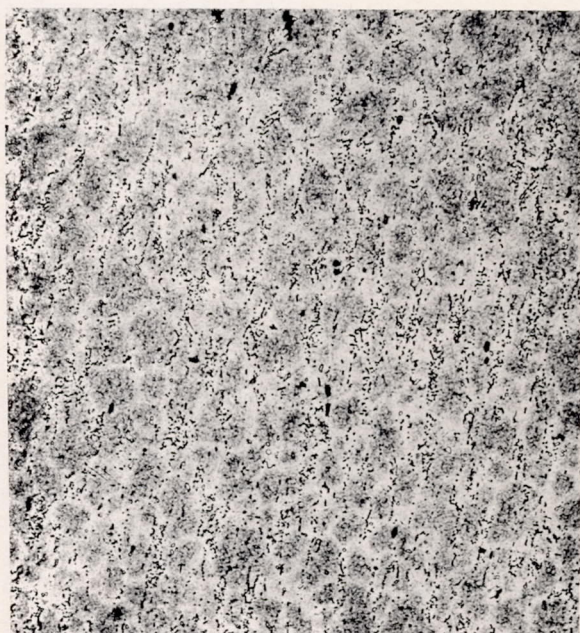
(a) Specimen 13Z; 1002 hours at 1200° F under 35,000 psi.
