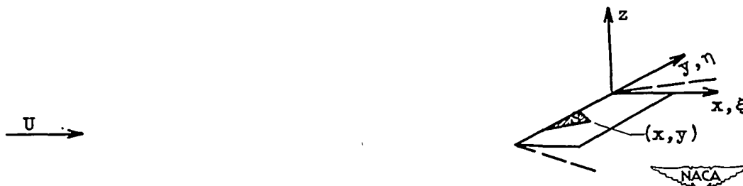
(c) Potential \phi''' due to solution for tail surface in uniform stream.
