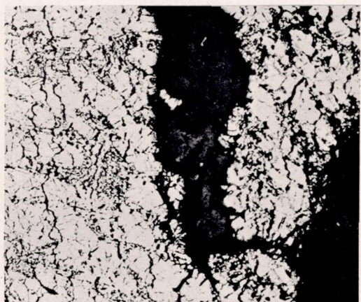
(b) Specimen F10A; 1894 hours for rupture at 1350° F and 27,000 psi.
