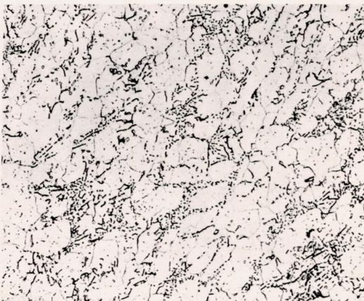
(c) Specimen Q5X; 2137 hours at 1500° F and 10,000 psi.
