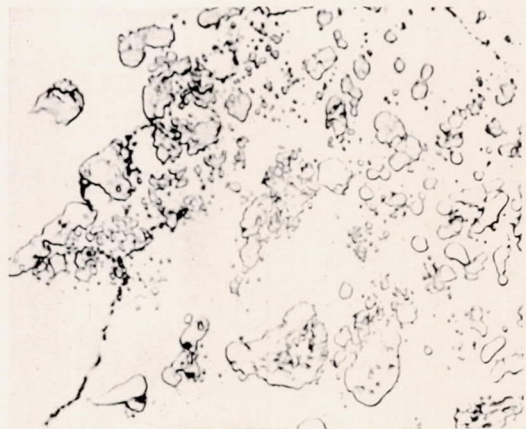
(a) Disc NR-76B-F; as-forged and aged. Radial section of Y-specimen near rim.
