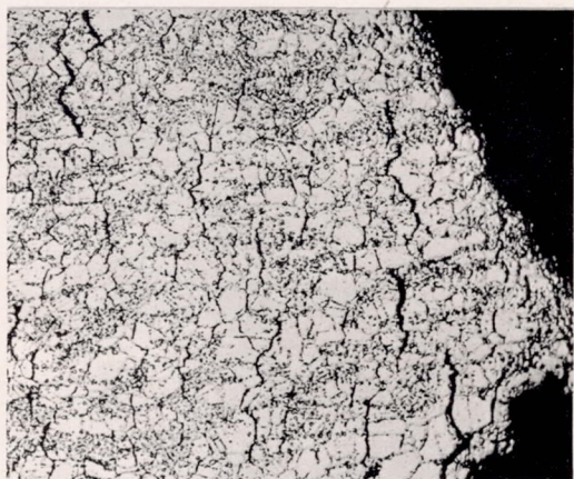
(a) Specimen F9A; 2618 hours for rupture at 1200° F and 45,000 psi.
