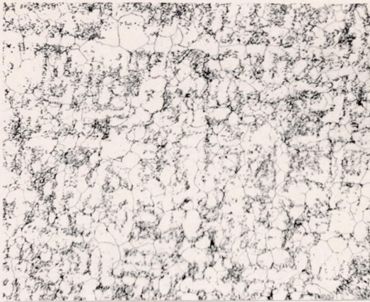
(a) Disc NR-76B-F; as-forged and aged. Radial section of Y-specimen near rim.
