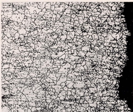
(a) Specimen F9A; 2618 hours for rupture at 1200° F and 45,000 psi.
