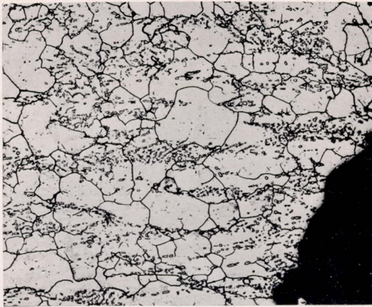
(a) Specimen Q12E; 1699 hours for rupture at 1200° F and 50,000 psi.
