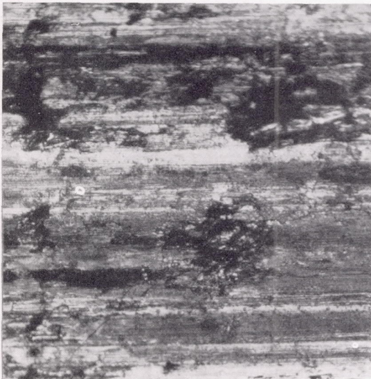
(c) Wear surface on rider containing 15-percent molybdenum disulfide \text{MoS}_2 , 80-percent silver Ag, and 5-percent copper Cu.
