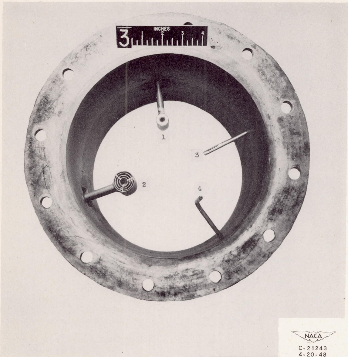
Figure 6. - Test section 3; (1) heated-shield thermocouple, (2) multiple-shield thermocouple, (3) Bureau of Standards gold-shield thermocouple, (4) pitot-static tube.
