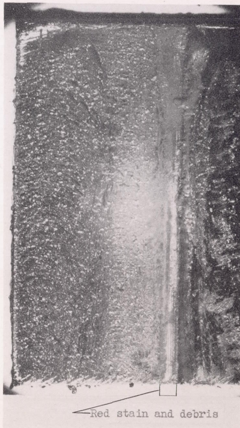
Figure 7. - Macrograph showing fretting corrosion caused by vibrating blue Swedish spring steel coated with mixture of molybdenum disulfide and heavy grease in contact with clean steel for 1,620,000 cycles. X5.
