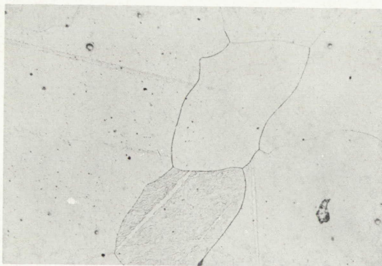
Figure 24.- Photomicrograph of M1 alloy (0 percent cerium and 1.80 percent manganese) in heat-treated, quenched, aged, and stabilized condition at a magnification of 250X. Heat, A4993-X6; minimum creep rate at 600° F and a 2000-psi stress, 0.0003 percent per hour; deformation in 120 hours, 0.090 percent; duration of test, 607 hours; final total deformation, 0.281 percent. (Similar to fig. 23. The cause of better creep resistance is probably a finer distribution of the manganese phase, but this is not revealed by metallography up to 500X.)
