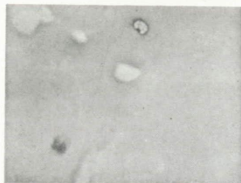
Figure 35.- Electron micrographs of an extruded alloy containing 2.33 percent cerium and 0 percent manganese in heat-treated, aged, and stabilized condition at a magnification of 5000X. Specimen, A5107. (This sample was not tested in creep; it was used to establish a base line for comparison with the cerium-manganese alloys. Specimen A5107-X5, which was tested in creep, is a duplicate of this bar.)
