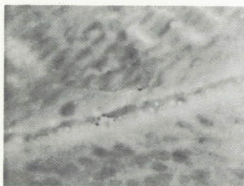
Figure 37.- Electron micrographs of extruded EM22 alloy (2.41 percent cerium and 1.90 percent manganese) in annealed condition at a magnification of 5000X. Specimen, A4975-X8; minimum creep rate at 600° F and a 2000-psi stress, 0.175 percent per hour; duration of test, 51 hours; final total deformation, 11.04 percent. (Sample was taken from stressed portion of creep test specimen.)
