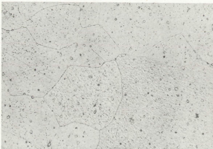
Figure 27.- Photomicrograph of an alloy containing 1.34 percent cerium and 1.56 percent manganese in heat-treated, aged, and stabilized condition at a magnification of 250X. Heat, A5110-X5; minimum creep rate at 600° F and a 2000-psi stress, 0.0014 percent per hour; deformation in 120 hours, 0.303 percent; duration of test, 597 hours; final total deformation, 1.05 percent. (Shows small particles of cerium-rich phase.)
