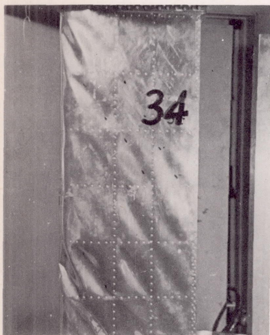
(c) Failure produced by collapse of nose section.
