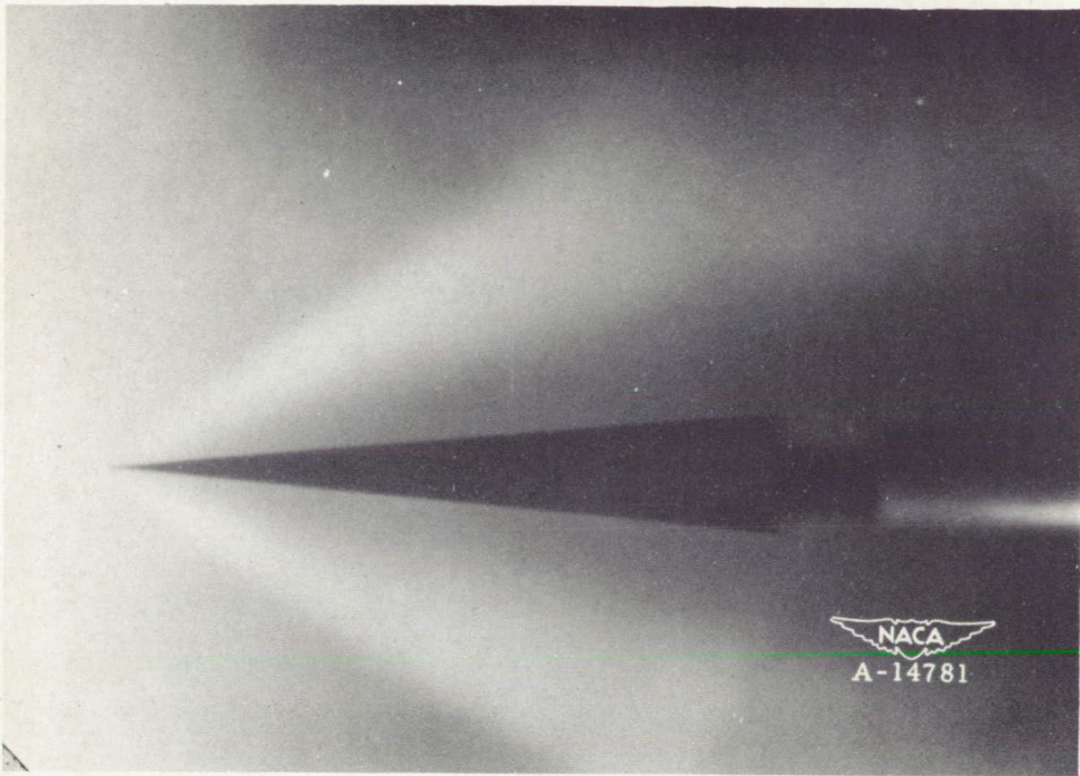
Figure 15.— Shock wave from 5^\circ half-angle wedge at pressure of 114 microns as seen with nitrogen glow discharge.
