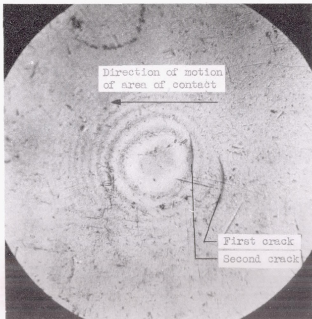
(b) View of ball through glass showing second crack being formed in glass on trailing edge of area of contact.
