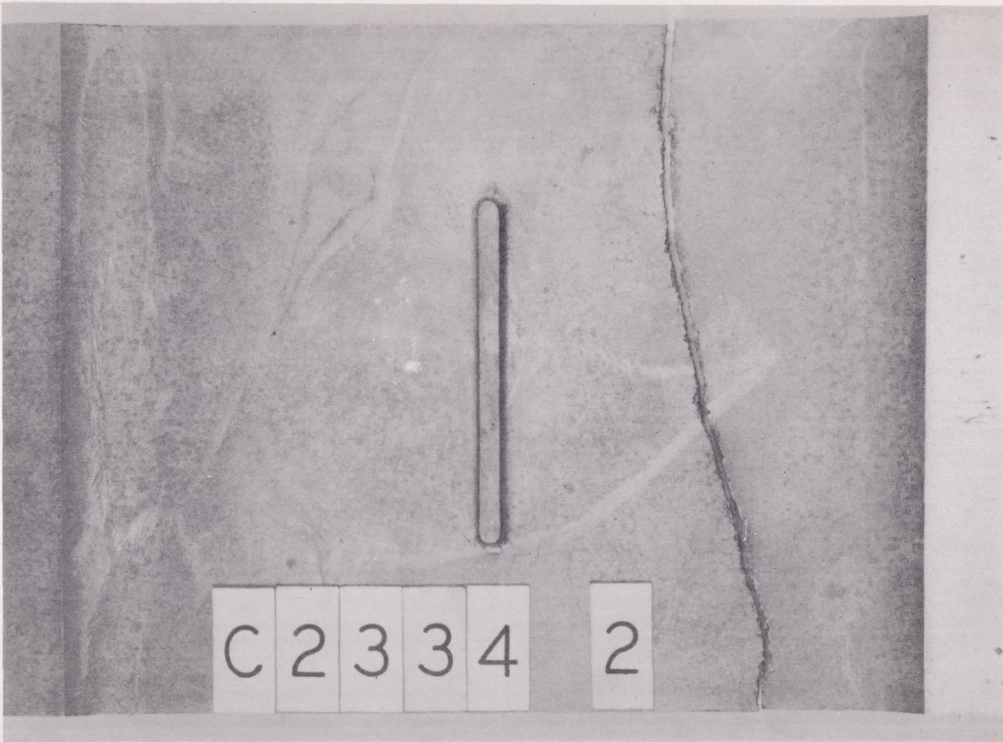
Figure 17.- Failure in type 5 specimen between rib and end of reduced section.
