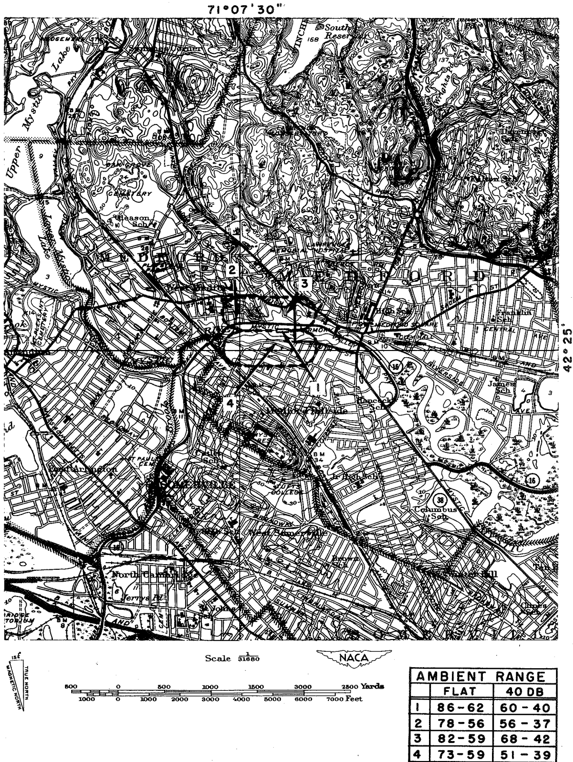
(b) Topographical map of surrounding area with air traffic pattern and ambient levels indicated.
