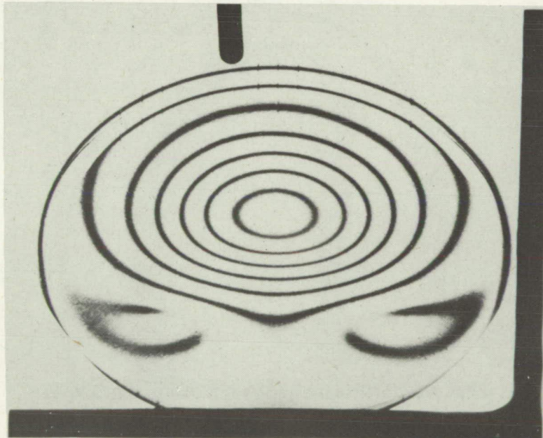
Figure 12.- Stress pattern of slice parallel to equator at normal incidence.
