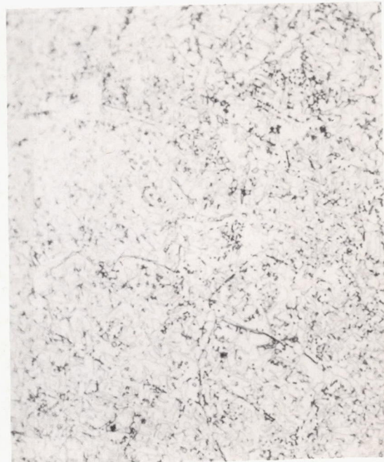
(a) Chromium, 10 percent (heat 51); 318 hours for rupture under 12,000 psi.
