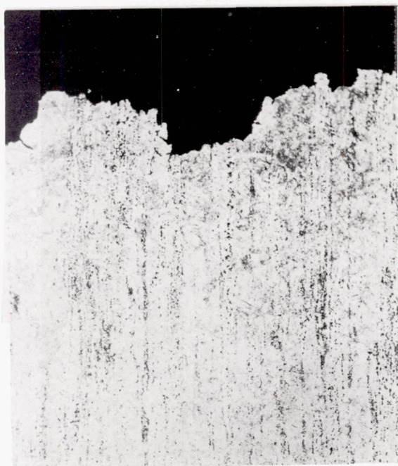
(a) Carbon, 0.08 percent (heat 13); 328 hours for rupture under 13,000 psi.
