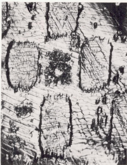
(a) Time, 1 hour; temperature, 600^{\circ}\text{C} ; stress, 100 psi; \alpha = 42^{\circ} , \beta = 43^{\circ} . X180.
