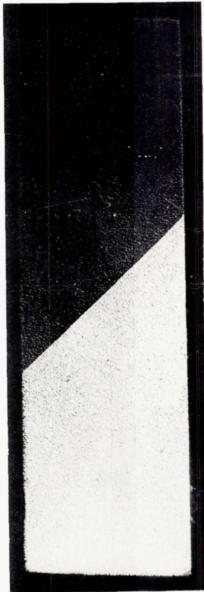
Figure 4.- Typical bicrystal cut, with grain boundary at 45^\circ , from coarse-grained aluminum plate. Tucker's etch. X4.
