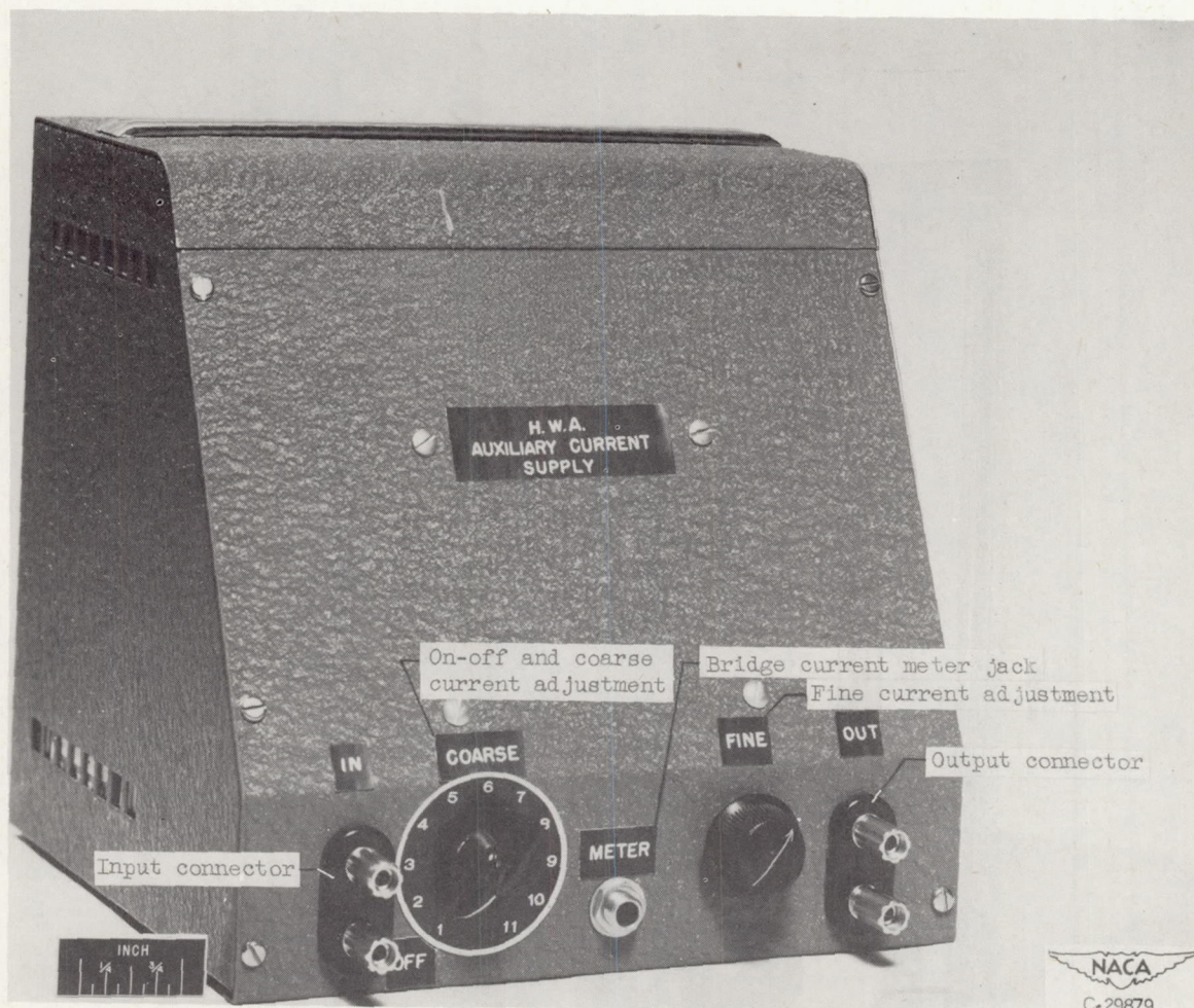
Figure 31. - Auxiliary current supply.
