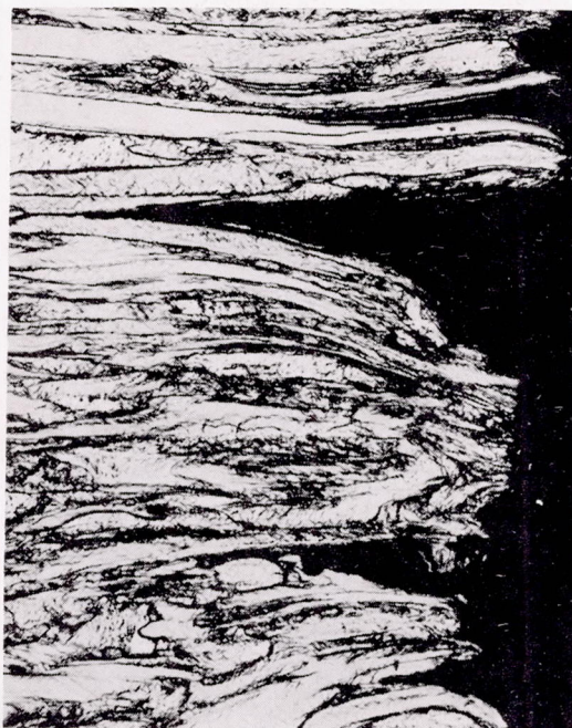
(b) Recrystallized; fractured at 325° F; 45 percent elongation.
