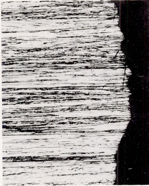
(a) As-swaged; fractured at -100^{\circ} F; 4.3 percent elongation.
