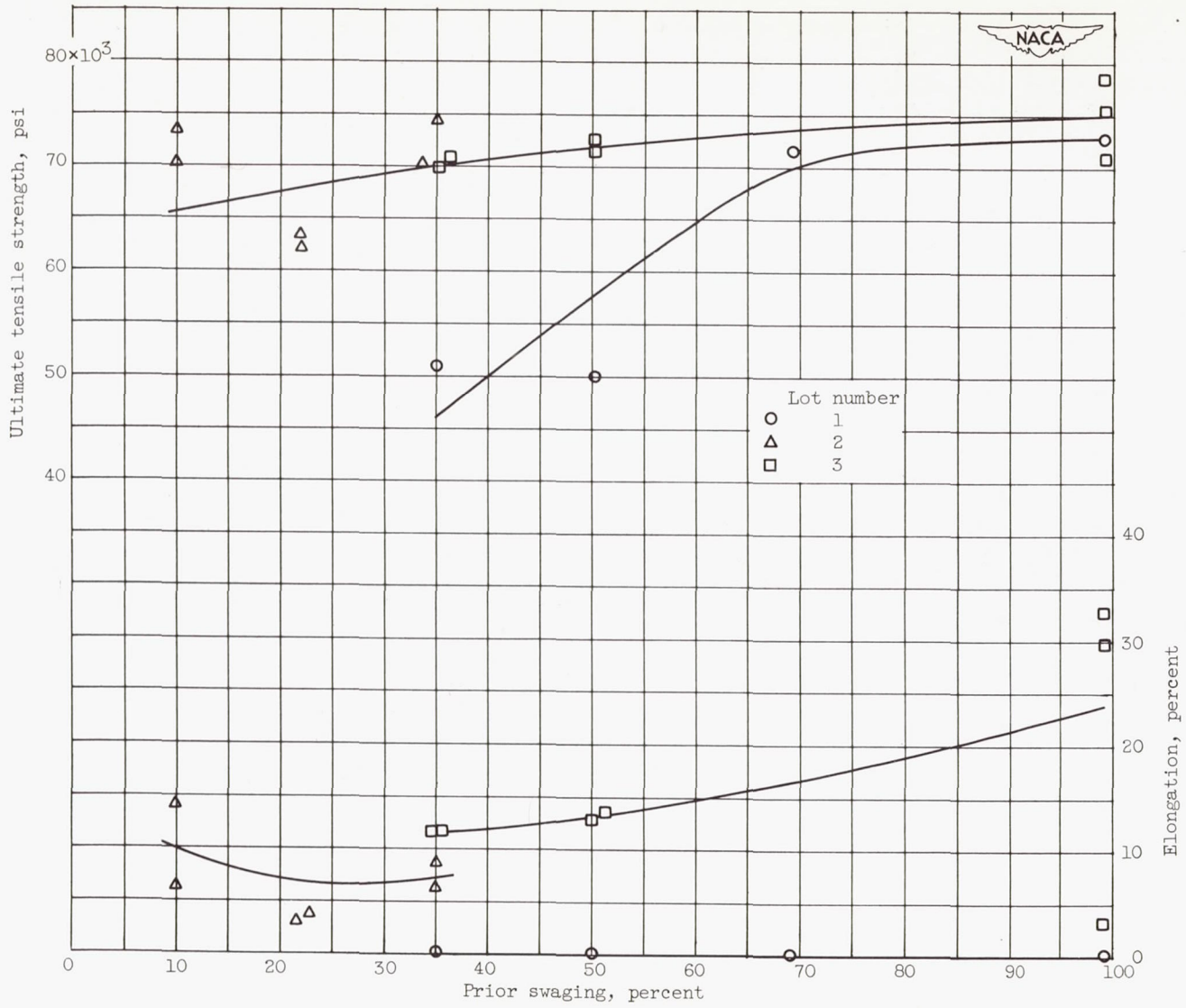
Figure 10. - Effect of prior swaging on room-temperature strength and ductility of recrystallized molybdenum.
