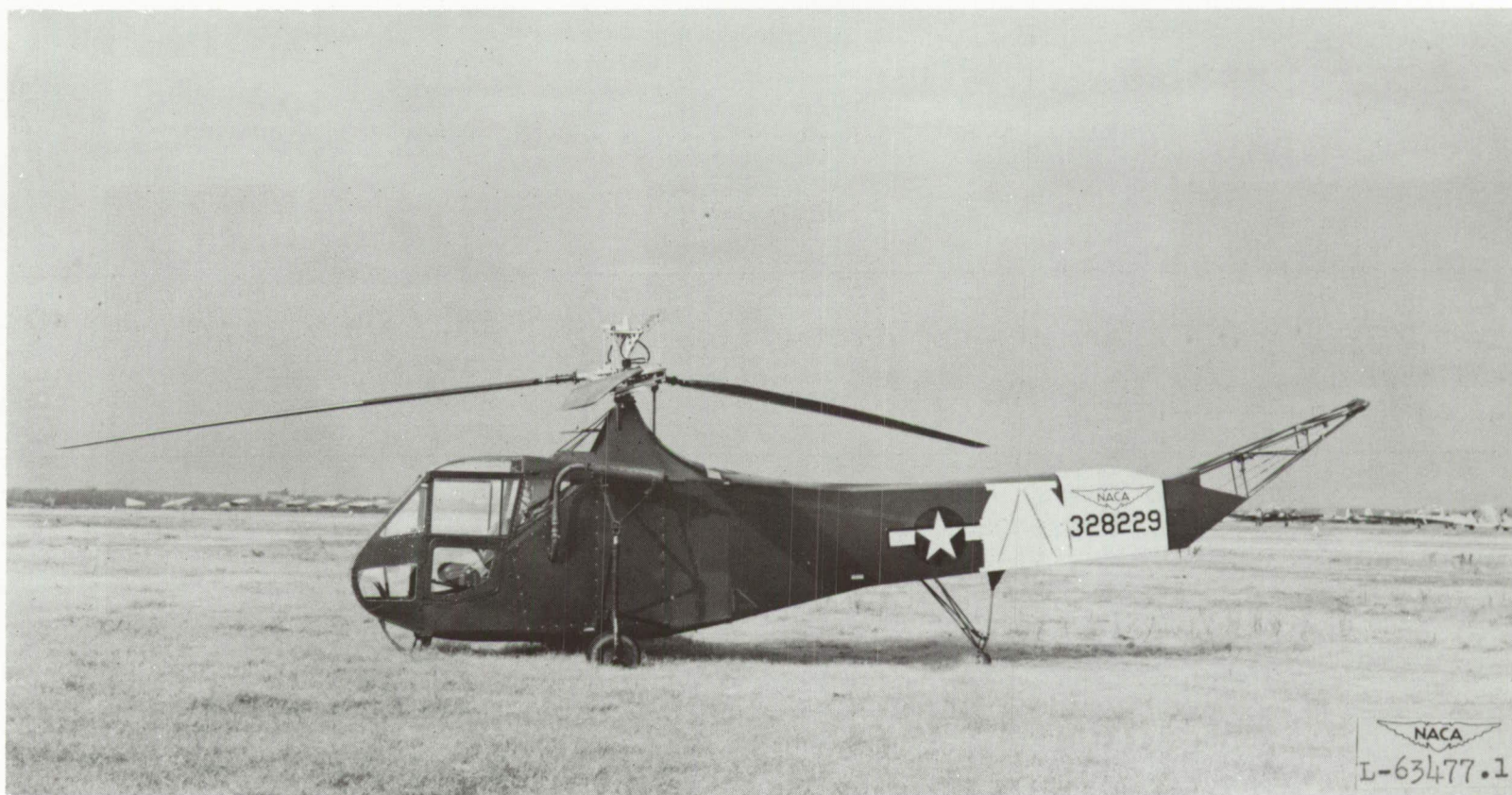
Figure 4.- Muffler 2 installed on helicopter with tail rotor removed.
