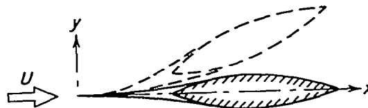
Sketch (d).- Smoothing for airfoil oscillating about leading edge.
