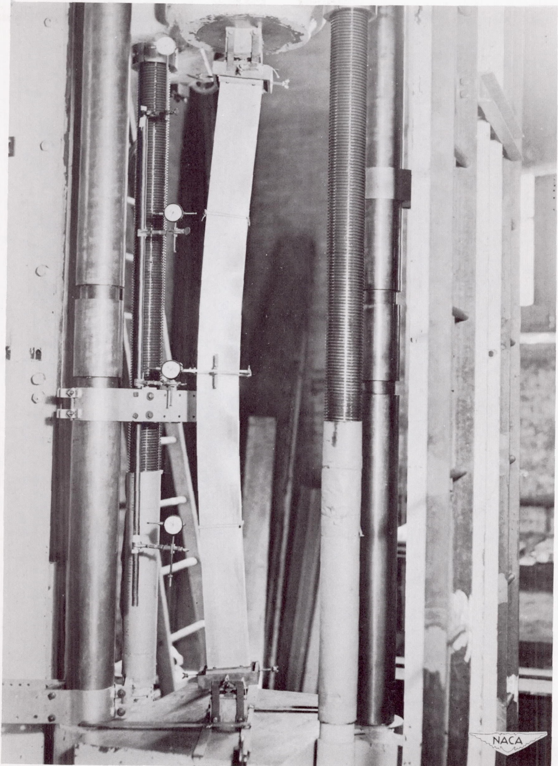
Figure 20.- View of test setup. Column shown is L3-M12.
