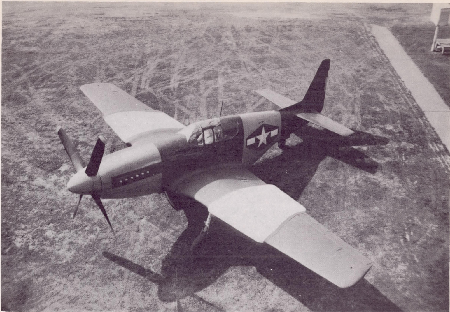
Figure 1.- Airplane with airfoils installed on left and right wings (prior to covering test-airfoil surfaces with aluminum sheets).
