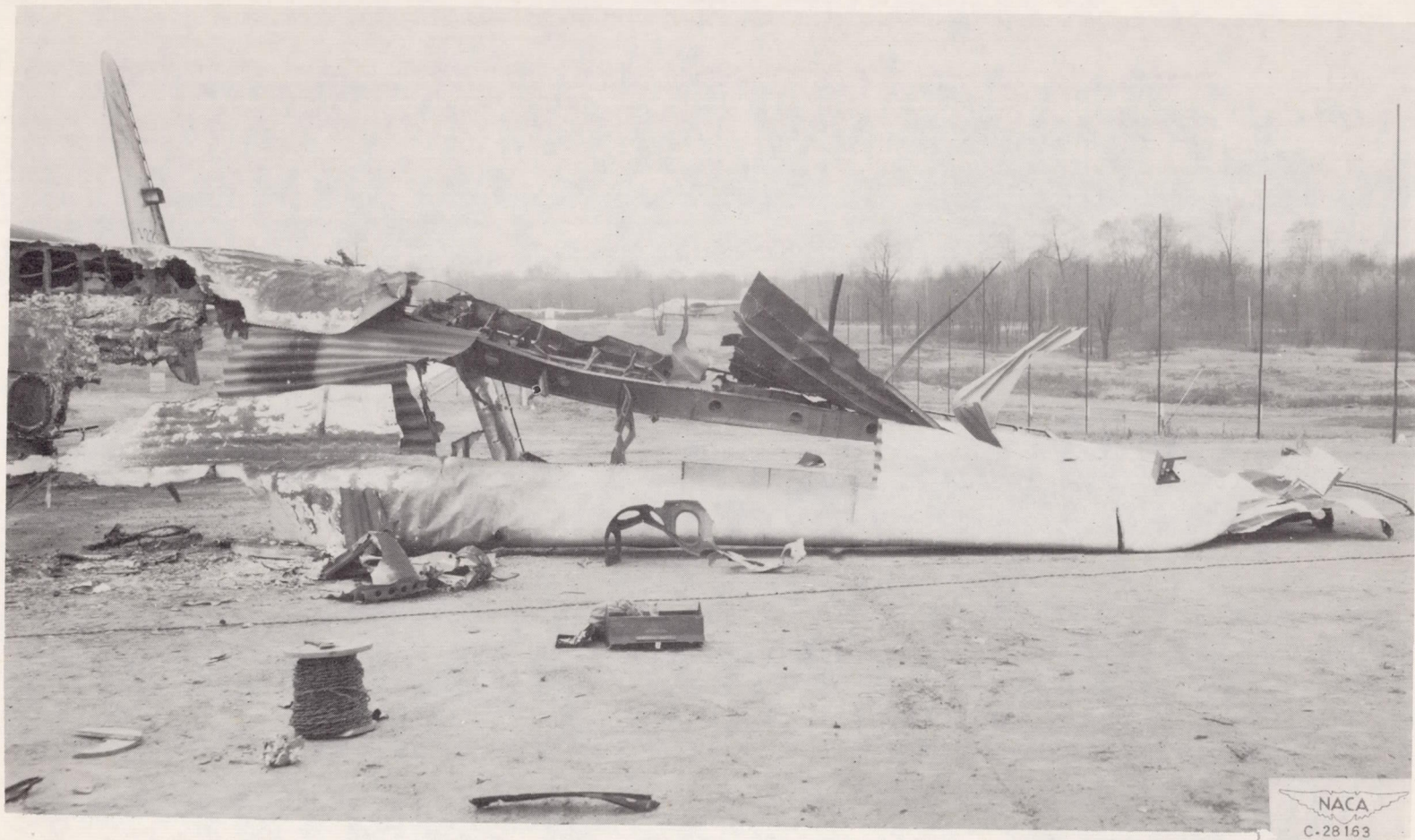
(c) Front view of damage to wing structure.
