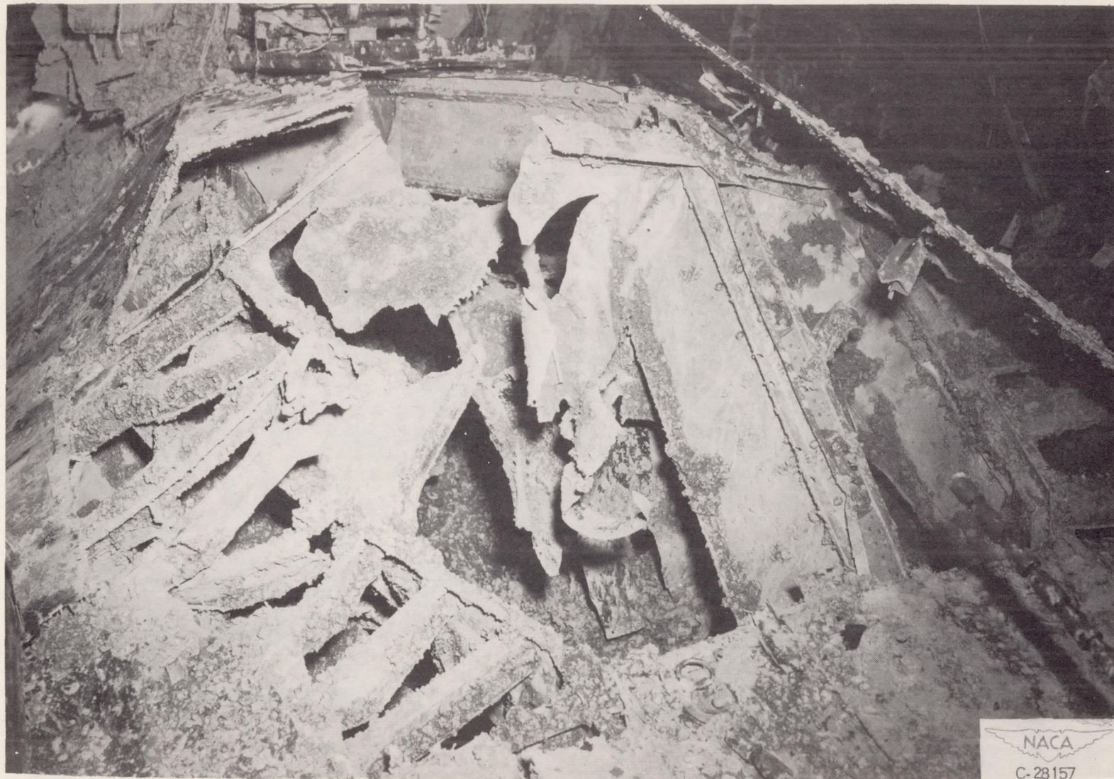
Figure 32. - Damage resulting when front landing-gear structure penetrates floor.
