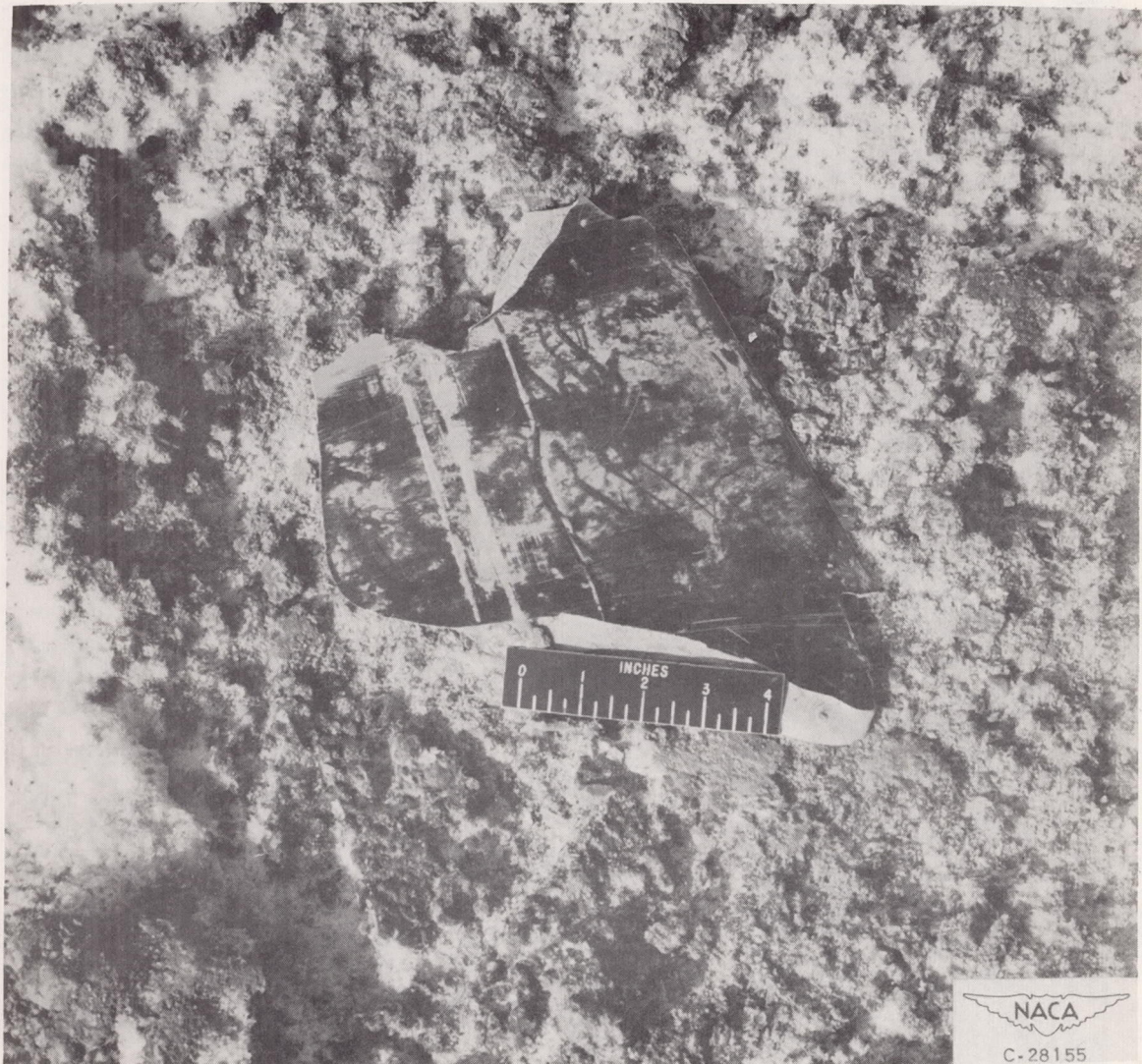
Figure 27. - Section of broken forged aluminum propeller blade caused by impact of blade with an obstacle.
