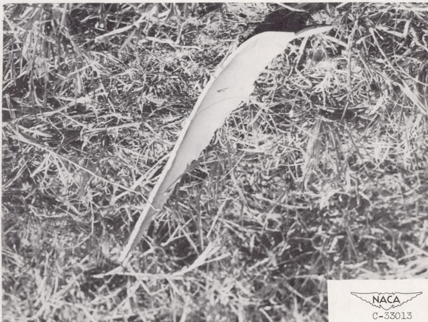
Figure 37. - Fragment of hydraulic shock strut cylinder found 150 feet from airplane after shock strut exploded because of fire.
