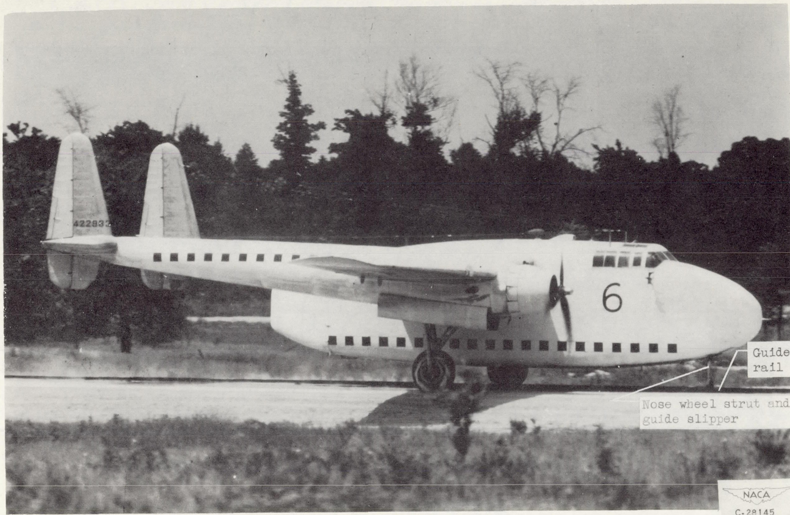
Figure 3. - Airplane with tricycle landing gear traveling along crash strip showing guide slipper attached to strut and replacing nose wheel.
