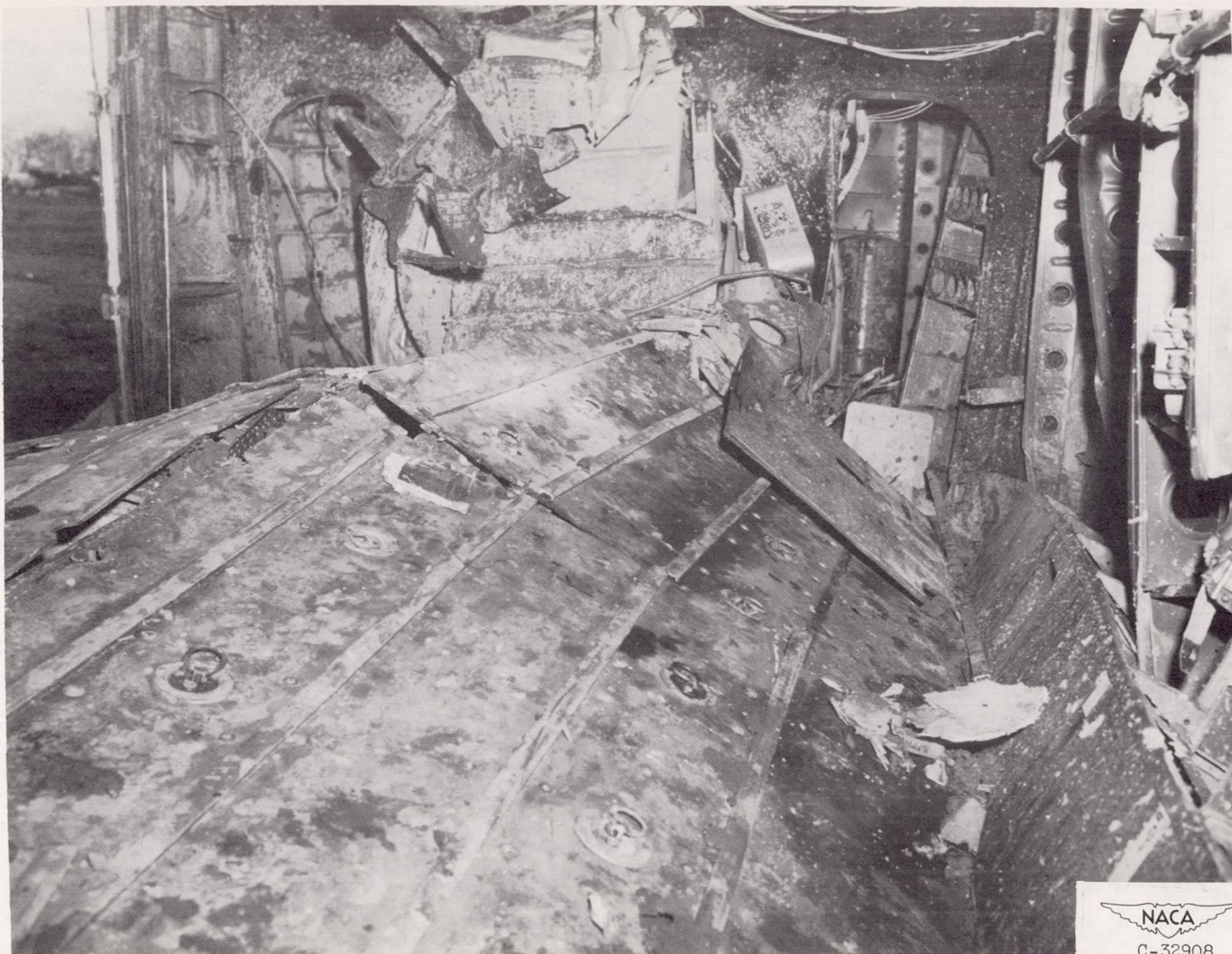
Figure 41. - Floor structure of cargo-type airplane severely damaged and bulged upward as a result of nose-wheel damage and landing upon a mud surface.
