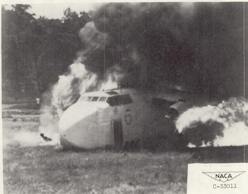
Figure 12. - Location of fire and wind direction such that fuselage is bathed in flame but pilot's compartment not enveloped.
