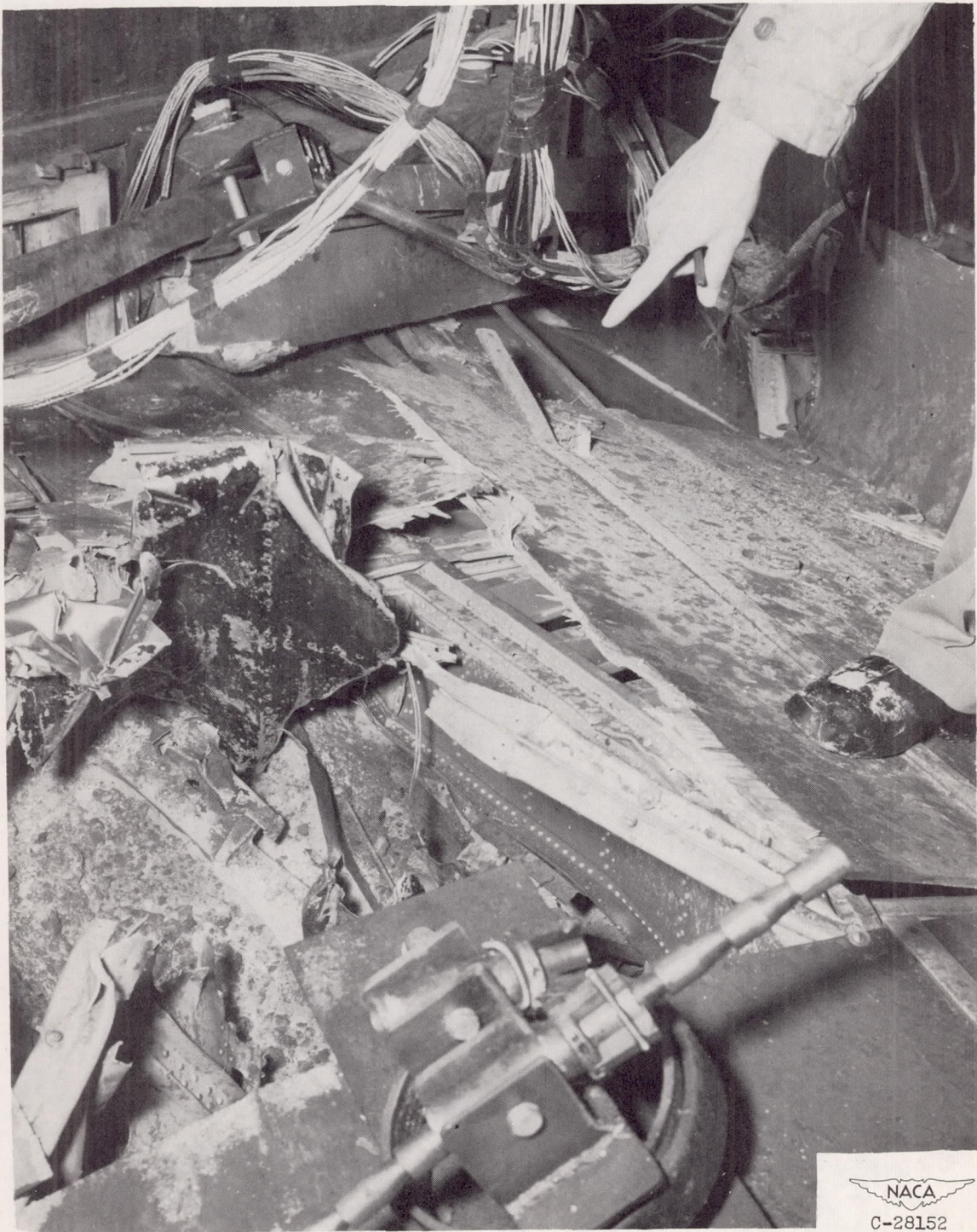
Figure 30. - Hole made in floor when front landing-gear strut and guide slipper were detached by contact with obstacle at crash barrier and penetrated floor structure.
