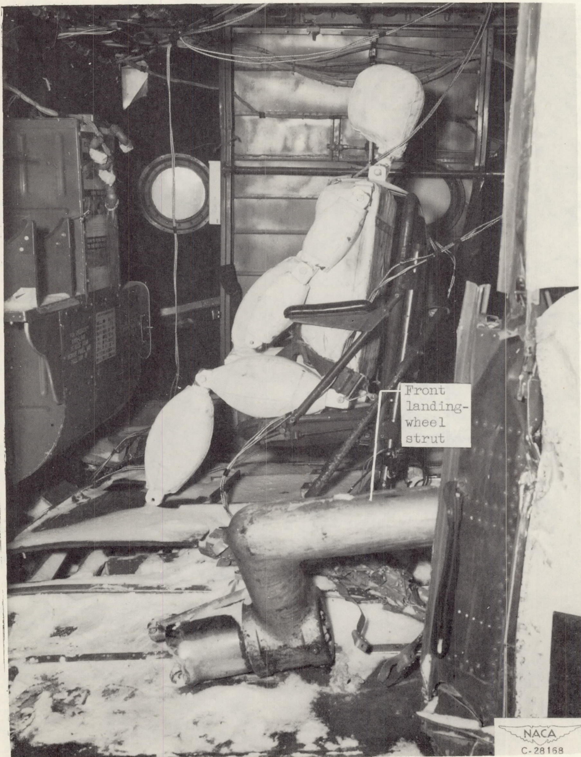
Figure 31. - Position of front landing-wheel strut after penetrating floor and rebounding from rear of cabin.
