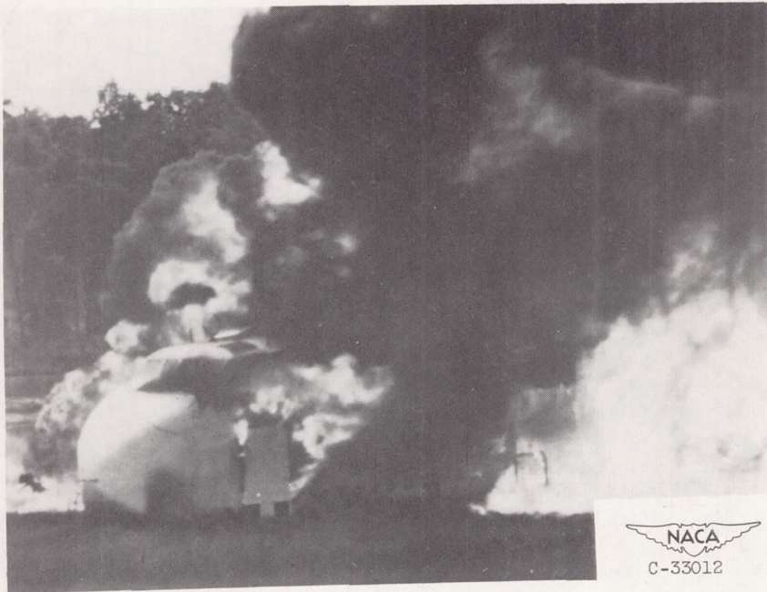
Figure 22. - Flame from explosion of hydrocarbon vapor in fuselage escaping through forward fuselage door.
