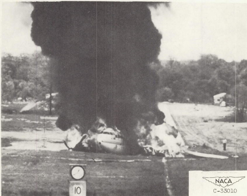
(b) Escape avenue to left front; wind from left rear quarter, variable at 0 to 5 miles per hour; crash 3.
