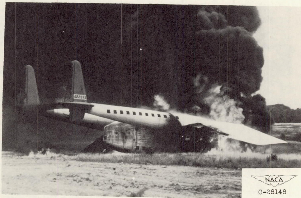
(e) Escape avenue to right rear after fuel mist fire burned away; wind from right rear, 10 to 15 miles per hour; crash 7.
