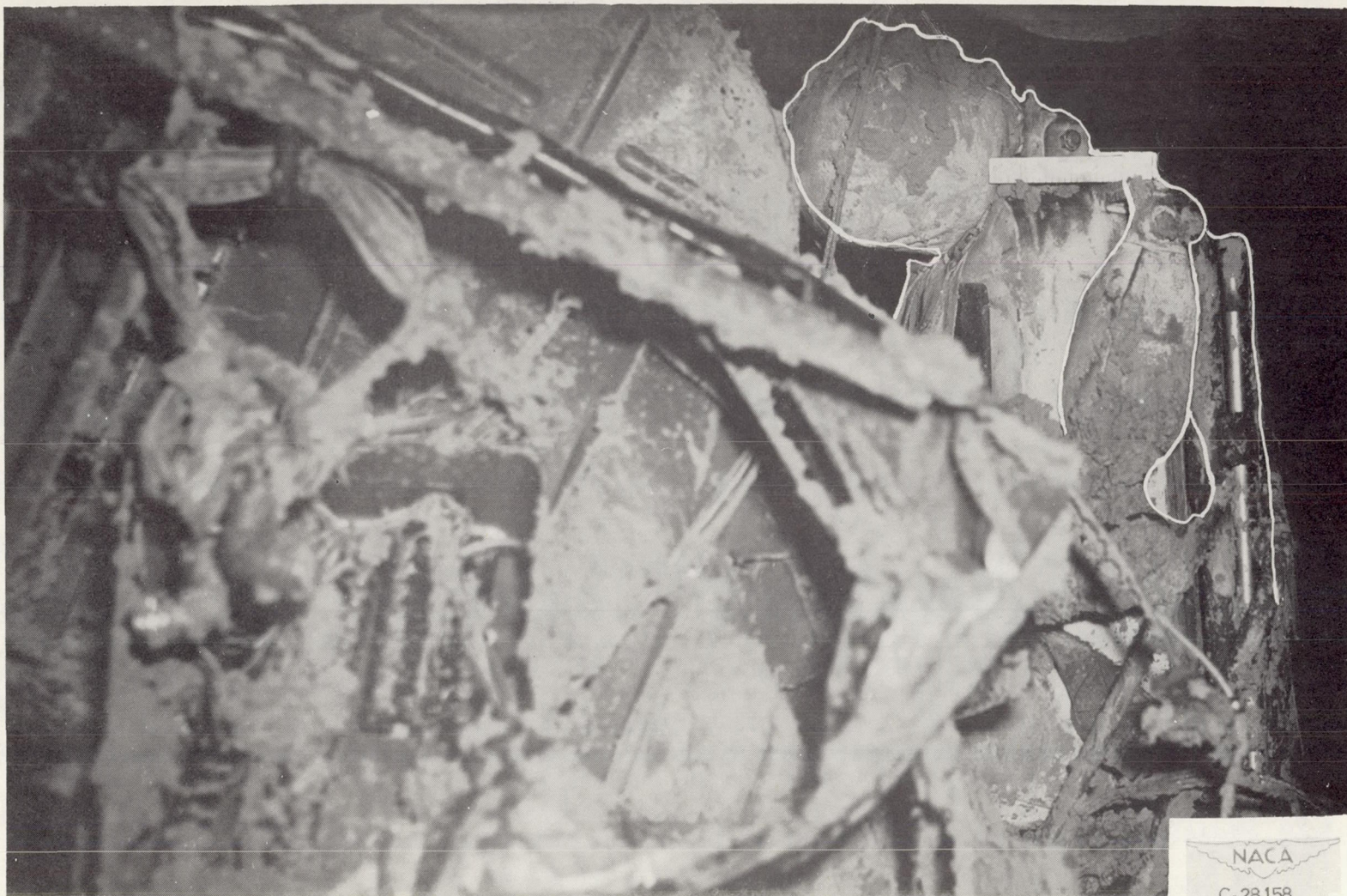
Figure 33. - Destruction of front landing-gear bulkhead and structure. Proximity to dummy shows possibility of injury to occupants seated in front part of fuselage.
