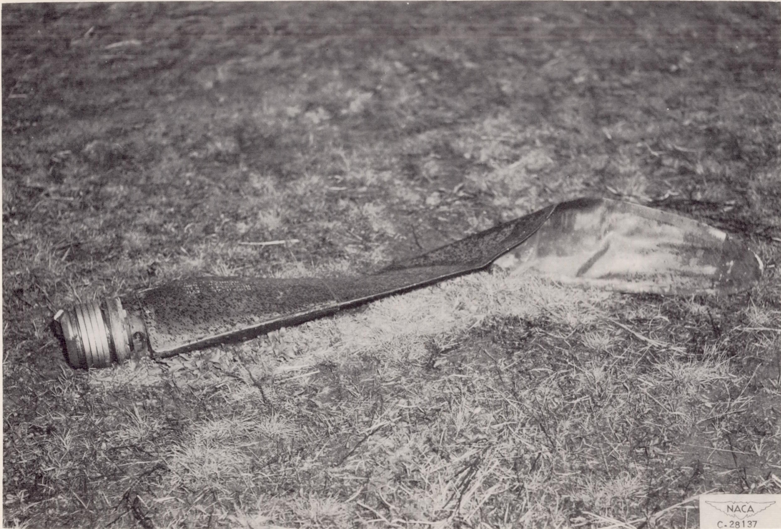
Figure 25. - Typical damage to steel propeller blade caused by impact with crash barrier.
