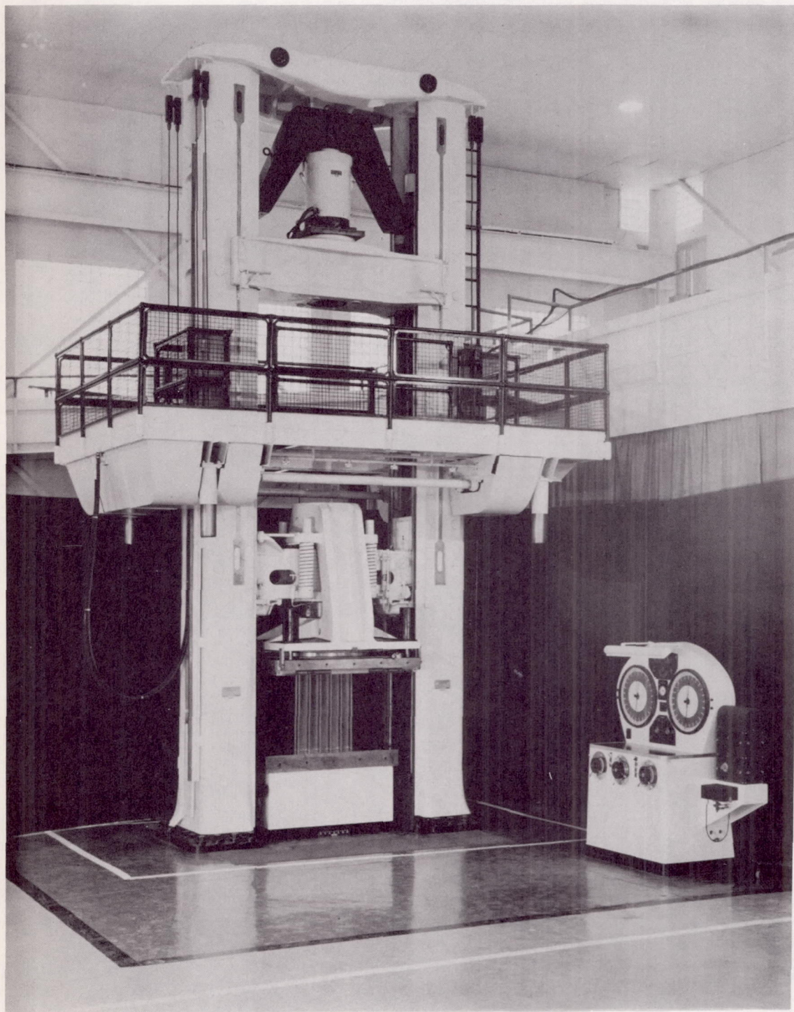
Figure 3.- Test set-up, showing jack and yoke arrangement at top of loading system to control crosshead motion beyond maximum load.
