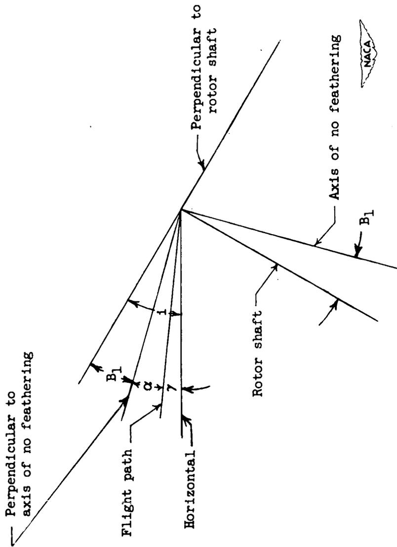
Figure 1.- Relation between rotor angle of attack, rotor-shaft incidence, angle of climb, and longitudinal cyclic pitch. All angles shown are positive. Axis of no feathering is uncorrected for blade and control-system distortion,  $\delta_3$ , or automatic control devices.
