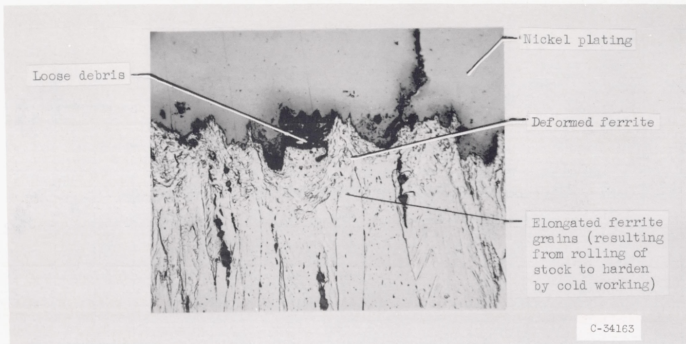
Figure 6. - Photomicrograph of taper section of fretted area of pure iron specimen fretted against pure iron for 400 cycles. Horizontal magnification, X500; vertical magnification, approximately X7500.
