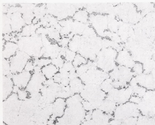
(d) Groups 18 to 26 (solution-treated and aged 72 hr at indicated temperatures).
