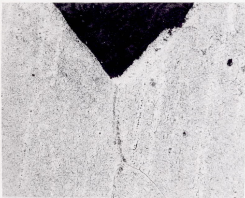
Solution-treated and "double-aged"; fractured after 168.6 hr at 21,000 psi
