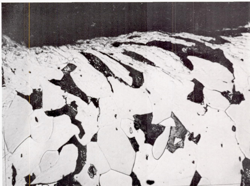
Figure 14.- Photomicrograph of mild steel surface fretted in air, X500. Pressure, 5,300 psi; frequency, 1,320 cpm; 0.0036-inch slip; 318,000 cycles.
