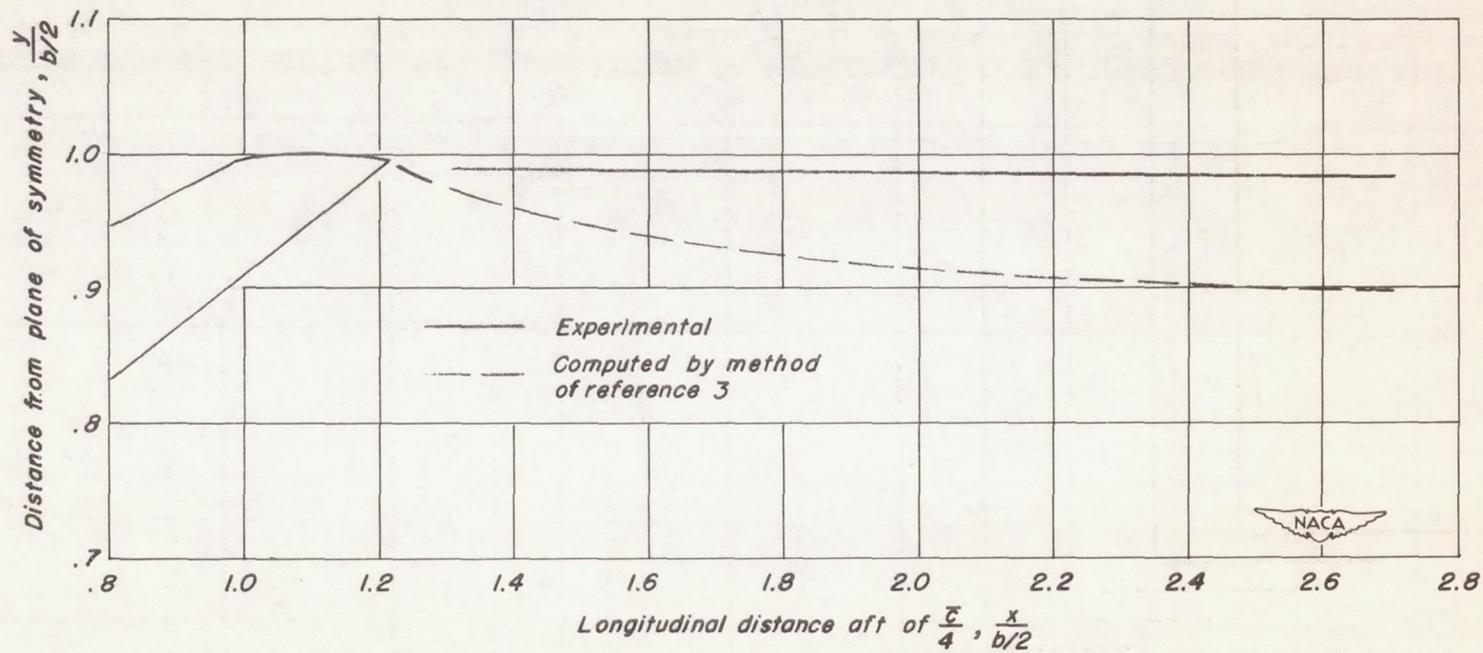
Figure 9.— Comparison of the experimental and computed tip vortex paths aft of the  $63^\circ$  swept-back wing-fuselage combination at  $\alpha = 12.3^\circ$ .
