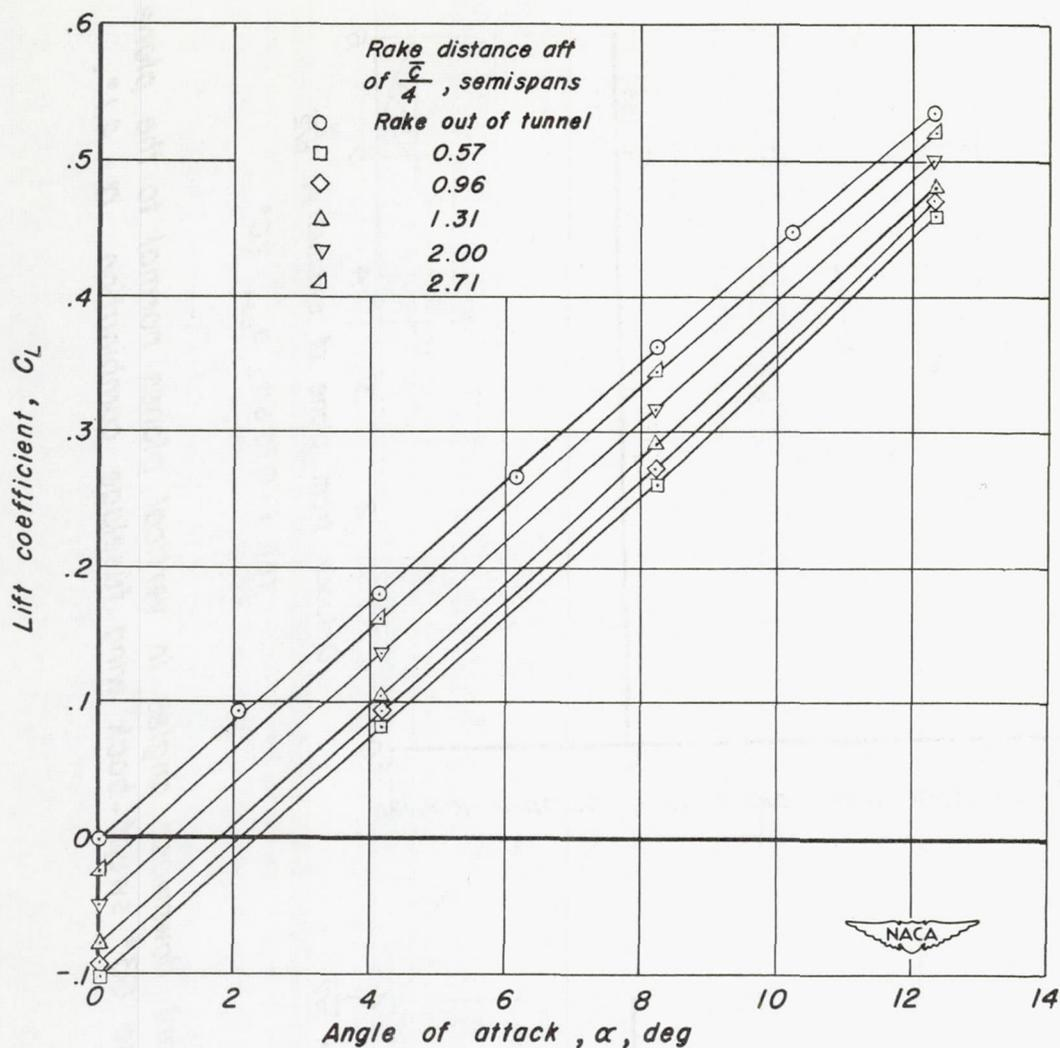
Figure 4.— Variation of lift coefficient with angle of attack for various longitudinal positions of the survey rake. Angle of attack corrected for tunnel-wall effect and flow inclination.
