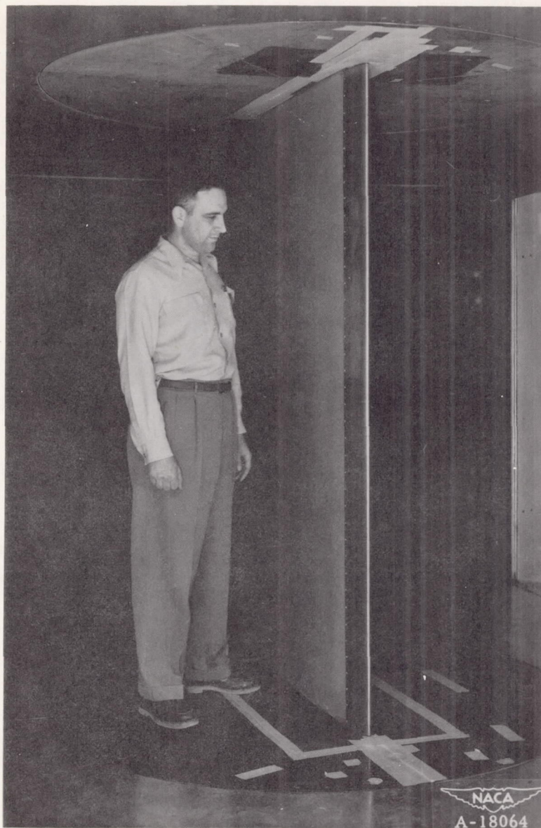
Figure 1.- The NACA 0006 airfoil with a porous leading edge.
