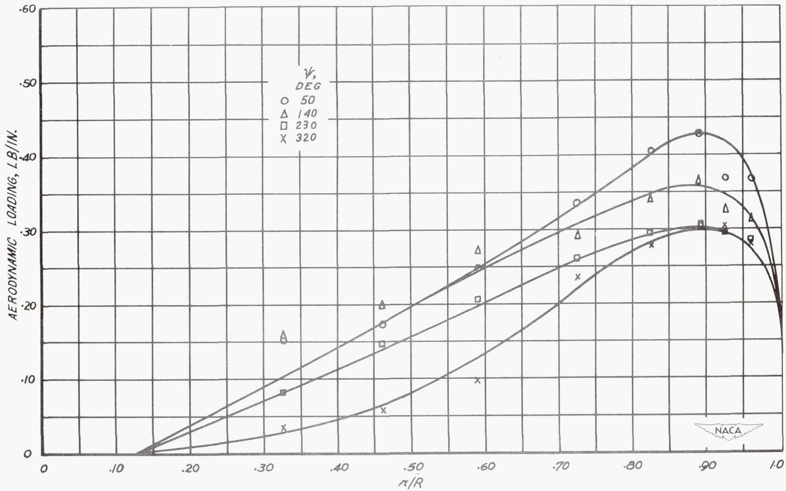
Figure 33.- Spanwise aerodynamic loading at various azimuth positions. Profile, NACA 0015; speed, 800 rpm; \xi = 0 ; \mu = 0.50 ; \theta = 8^\circ ; \alpha = -5^\circ ; C_T/\sigma = 0.076 .
