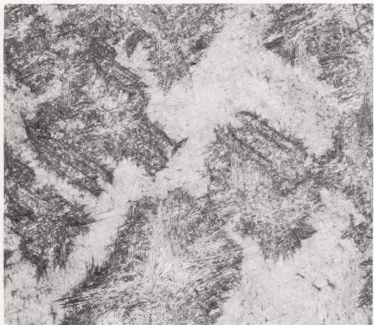
(c) Rolled 50 percent, showing islands of martensite-like NiAl; air quench; X100.
