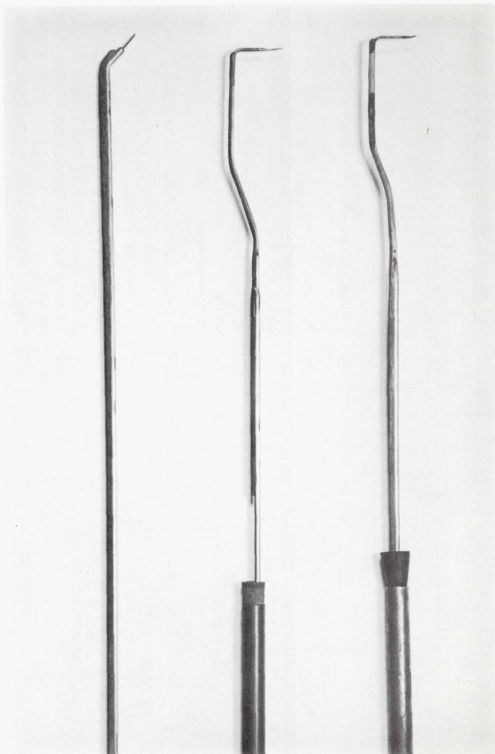
Figure 5.- Velocity measuring probes. From left to right, hot-wire, 0.019-inch outside-diameter boundary-layer impact tube, and 0.010-inch outside-diameter boundary-layer impact tube.
