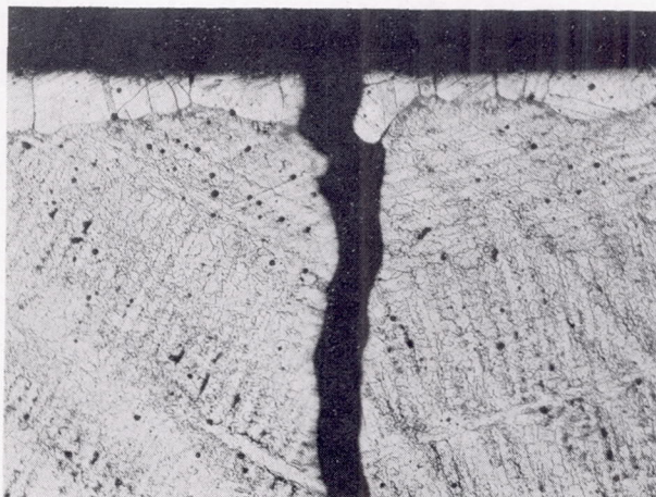
Figure 30. - Crack below fractured edge of blade from group 13. Electrolytically etched in 5 percent aqua regia.
