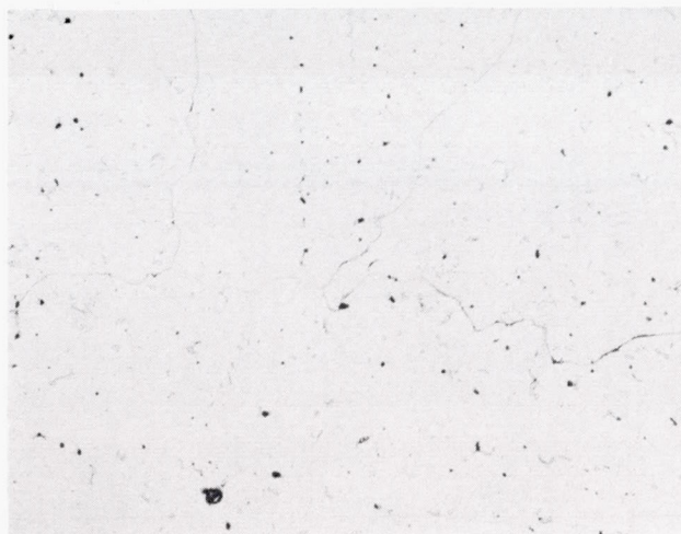
(b) Solution treated 24 hours at 2175° F and air cooled prior to aging (group 14).
