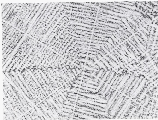
Figure 23. - Microstructure of cast HS-21 turbine blade solution treated 1/2 hour at 2150° F, air cooled, and aged 48 hours at 1500° F after operation for 196.13 hours at rated speed (group 3). Electrolytically etched in 5 percent aqua regia.
