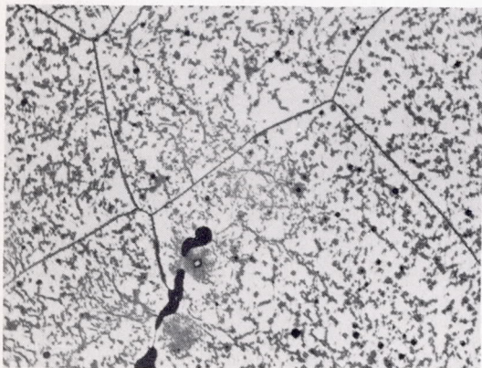
(c) Solution treated 72 hours at 2250° F and air cooled prior to aging (group 23).
