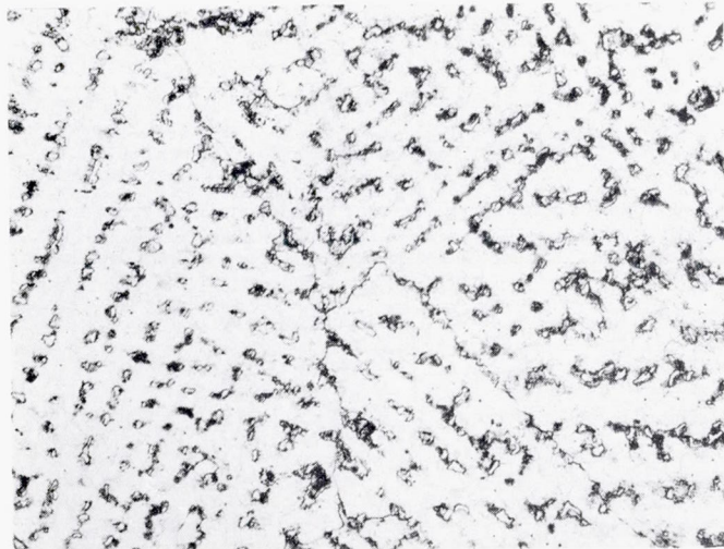
Figure 26. - Microstructure of cast HS-21 turbine blade solution treated 24 hours at 2050° F, air cooled, and aged 48 hours at 1200° F after operation 68.4 hours at rated speed (group 12). Electrolytically etched in 5 percent aqua regia.
