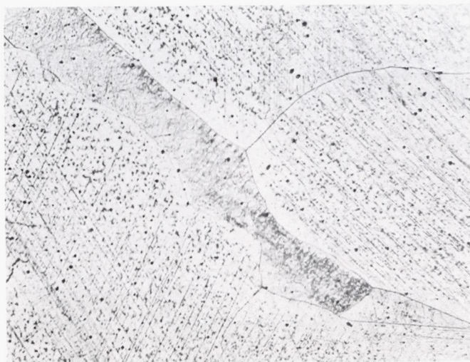
Figure 27. - Microstructure of cast HS-21 turbine blade solution treated 24 hours at 2175° F, air cooled, and aged 48 hours at 1200° F after operation 64.1 hours at rated speed (group 14). Electrolytically etched in 5 percent aqua regia.
