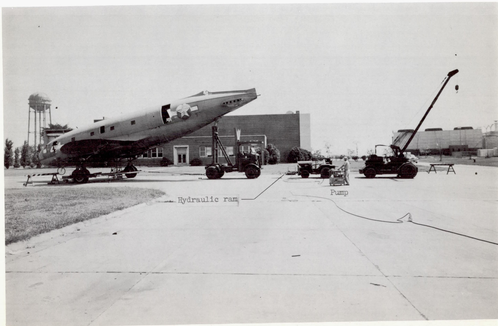
Figure 5.- Locked-wheel drag-test setup.
