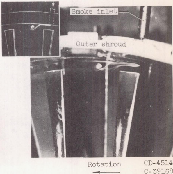
(c) Tip clearance, 0.023 inch; U/V_x , 1.25. (d) Tip clearance, 0.200 inch; U/V_x , 0.90.
