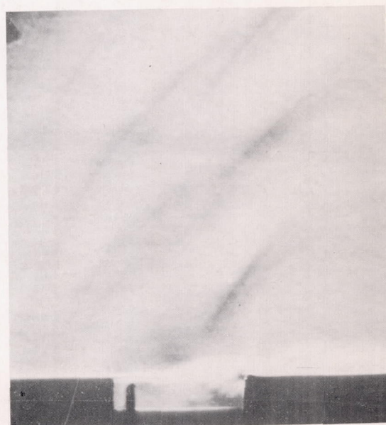
L-87930 (d) Gap with d = 0.1 inch and b = 0.4 inch. Knife edge horizontal.
