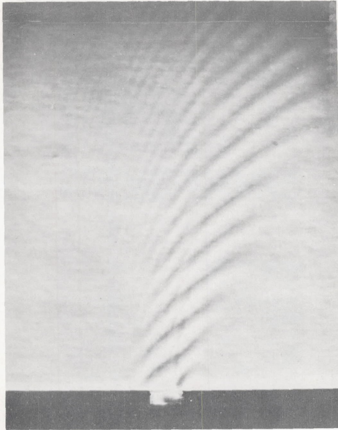
Figure 8.- Sound emission for gap 0.05 inch deep and 0.1 inch broad with laminar boundary layer. M_{\infty} = 0.854 ; T_0 = 116.8^{\circ} F.
