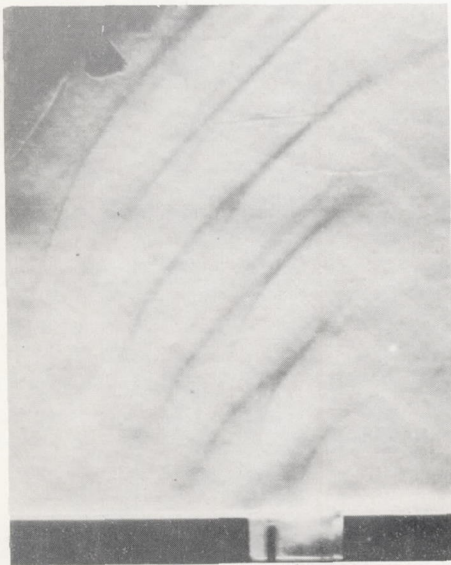
(a) M_\infty = 0.5 ; T_0 = 105^\circ \text{ F} . Knife edge vertical.
