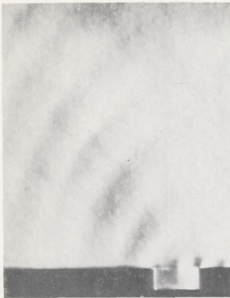
(a) M_\infty = 0.5 ; T_0 = 105^\circ \text{ F} . Knife edge vertical.
