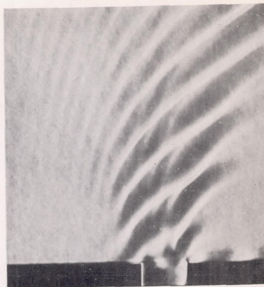
(b) Gap with d = 0.1 inch and b = 0.2 inch. Knife edge vertical.
