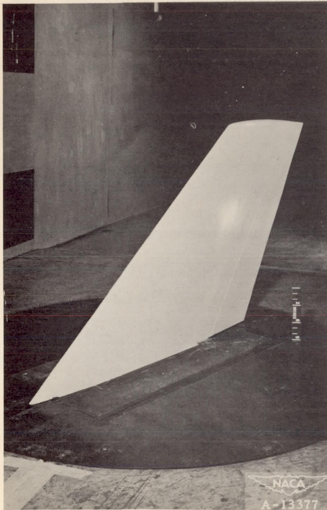
(a) The 45^\circ swept-back model of aspect ratio 2 in the 7- by 10-foot wind tunnel.
