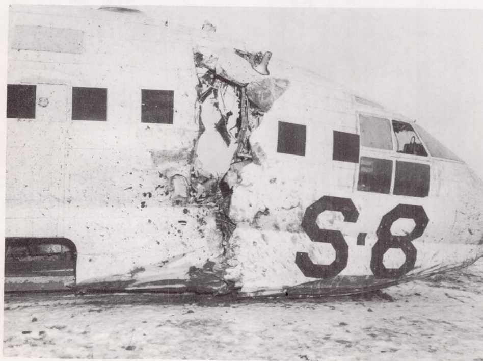
Figure 16. - Hole cut in fuselage by propeller blades.
