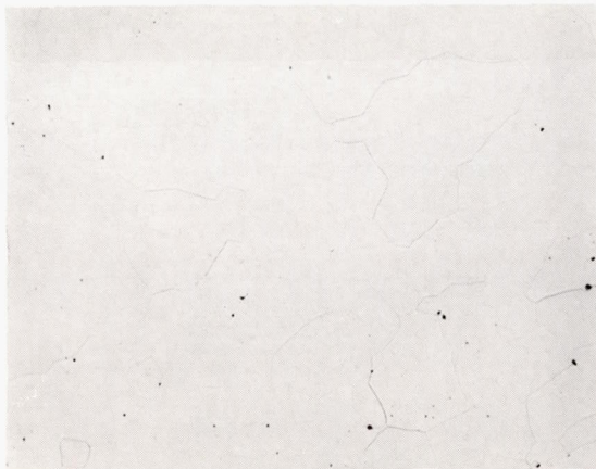
(c) 25-Percent-aluminum NiAl, homogenized at 2100° F for 48 hours.
