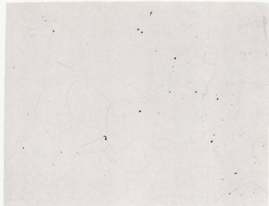
(b) 28-Percent-aluminum NiAl, homogenized at 2200° F for 48 hours.
