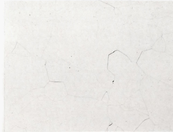
(b) 30-Percent-aluminum NiAl, homogenized at 2400° F for 6 hours.
