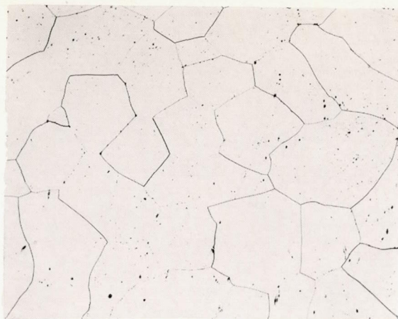
(a) 31.5-Percent-aluminum Al NiAl, homogenized at 2200° F for 48 hours.
