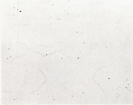
(a) 30-Percent-aluminum NiAl, homogenized at 2100° F for 48 hours.
