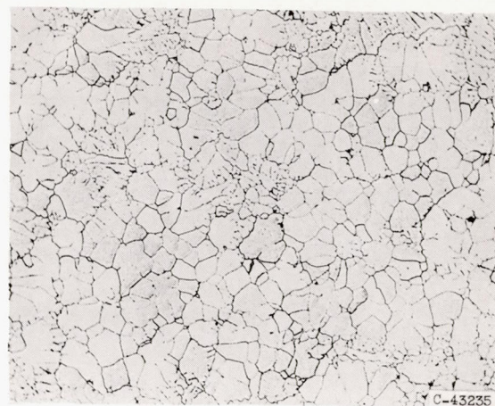
(d) 31.5-Percent-aluminum plus 2.0-percent-molybdenum NiAl, homogenized at 2300° F for 24 hours.
