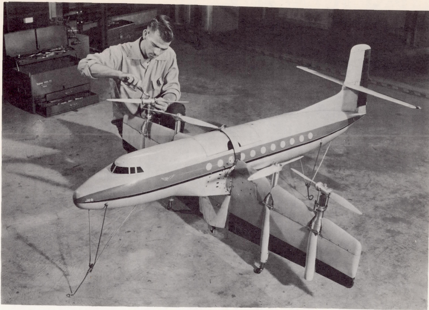
Figure 2.- Photograph of model in hovering configuration. Wing pivot located at 30 percent mean aerodynamic chord.
