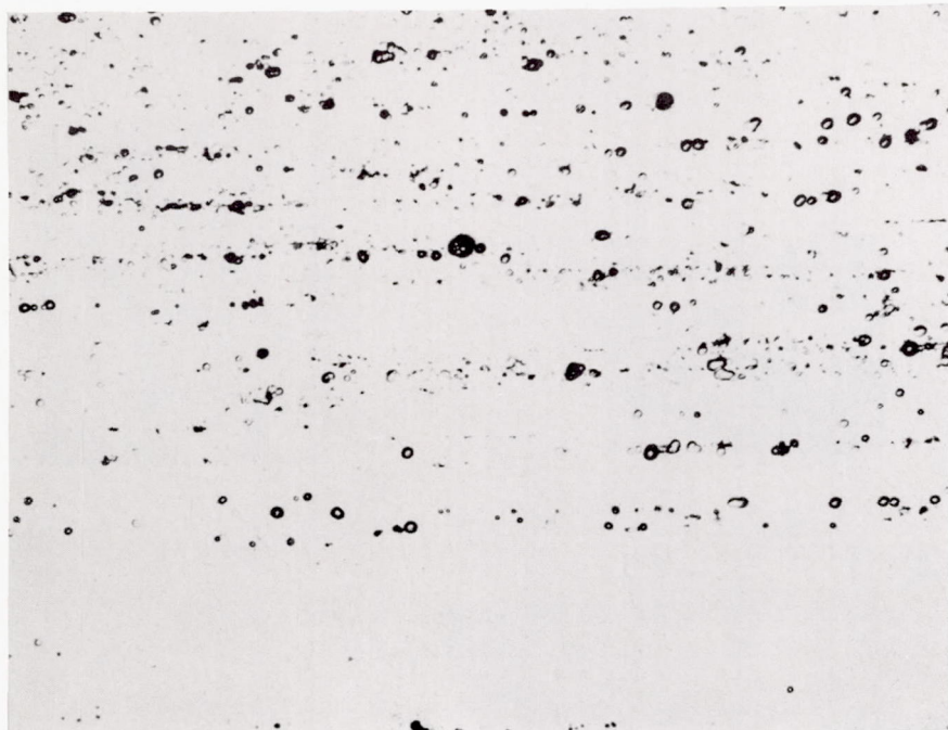
(f) Recrystallized longitudinal specimens. Unetched; 100X.
