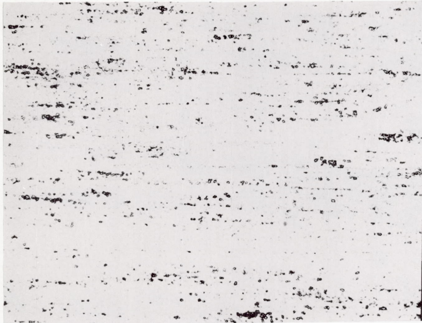
(e) Extruded longitudinal specimens. Unetched; 100X.
