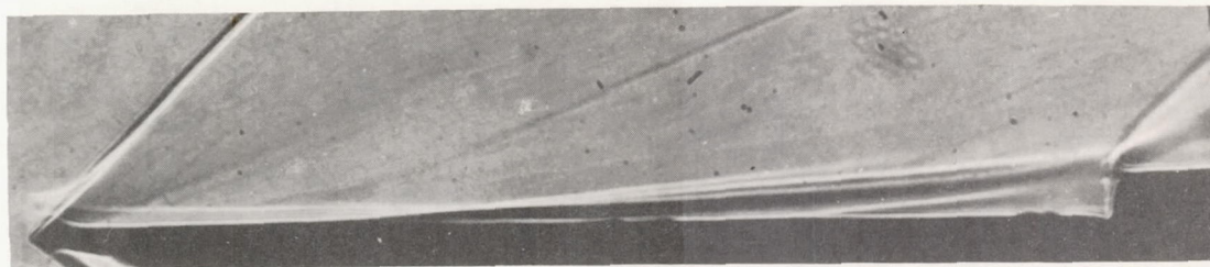
Figure 35.-Shadowgraph indicating lack of two-dimensional flow; S-3; M_0=3.0 ; R_L=0.57 \times 10^6 .
