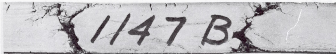
(b) Bar stock after reduction to 7/8-inch square. Large cracks occurred during ingot breakdown and could not be ground out.
